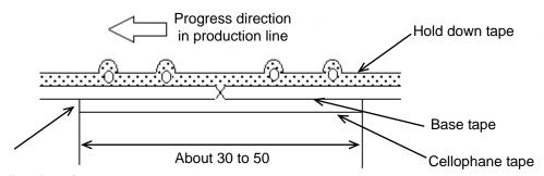
No lifting for the direction of progressing
