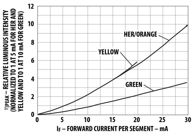
Figure 10. Relative Luminous Intensity vs. DC Forward Current.
