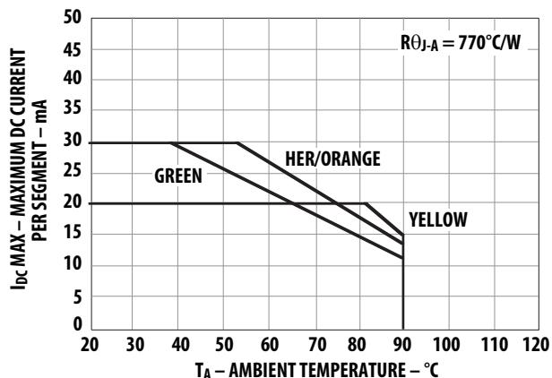
Figure 8. Maximum Allowable DC Current vs. Ambient Temperature.
