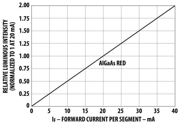
Figure 3. Relative Luminous Intensity vs. DC Forward Current.
