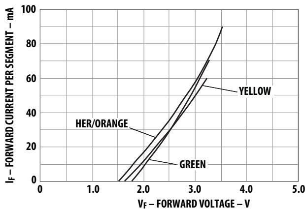
Figure 9. Forward Current vs. Forward Voltage Characteristics.
