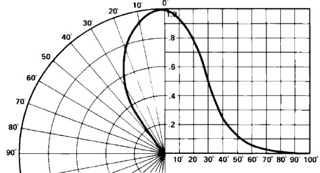
Figure 6. Relative luminous intensity vs. angular displacement.
