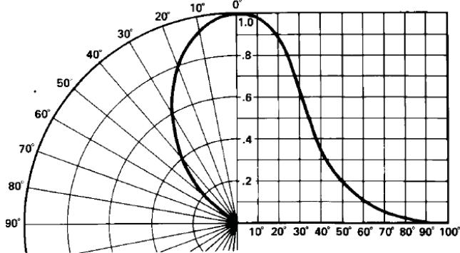
Figure 5. Relative luminous intensity vs. angular displacement.
