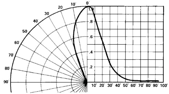
**Figure 8.** Relative luminous intensity vs. angular displacement.
