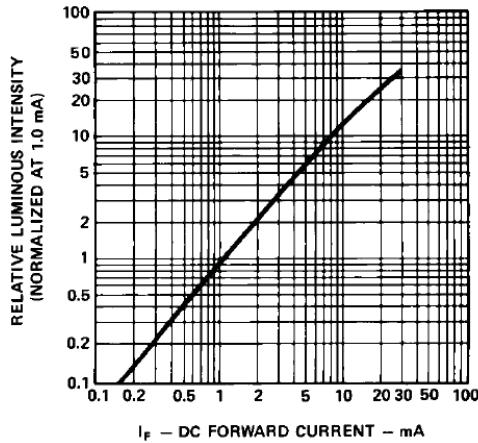
Figure 3. Relative luminous intensity vs. dc forward current.
