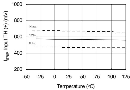
Figure 23A. I<sub>TRIP</sub> Input TH(+) vs. Temperature
