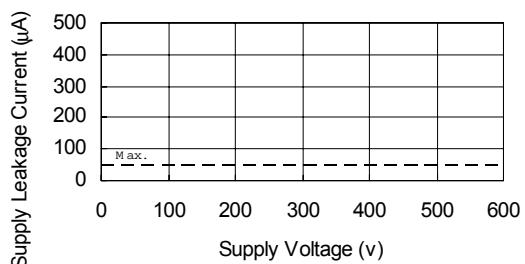
Figure 27B. Offset Supply Leakage Current vs. Voltage
