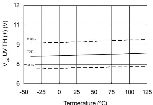
Figure 41B. IR2133/IR2233  $V_{cc}$  Undervoltage Threshold (-) vs. Temperature
