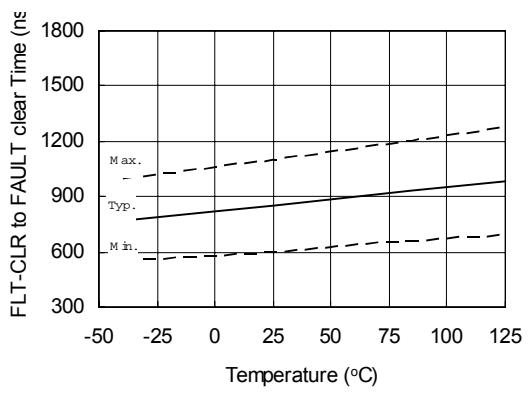
Figure 13A. FLT-CLR to FAULT clear Time
