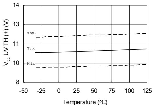
Figure 40A. IR2135/IR2235  $V_{cc}$  Undervoltage Threshold (+) vs. Temperature
