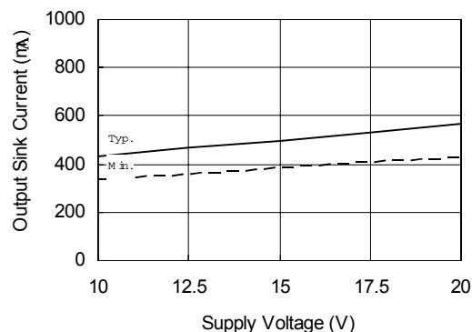
Figure 44B. Output Sink Current vs. Supply Voltage
