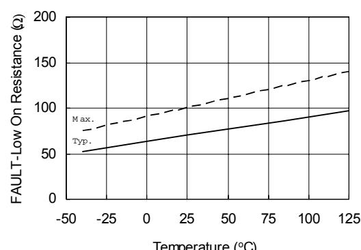
Figure 42A. FAULT- Low On Resistance vs. Temperature
