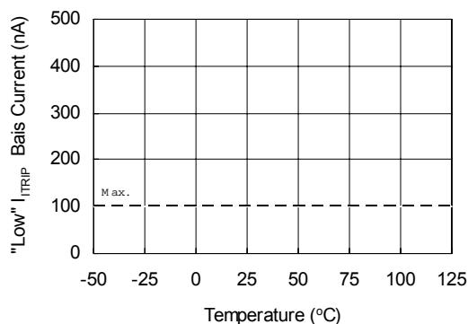
Figure 35A. "Low"  $I_{TRIP}$  Bias Current vs. Temperature
