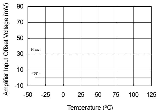
Figure 45A. Amplifier Input Offset Voltage vs. Temperature
