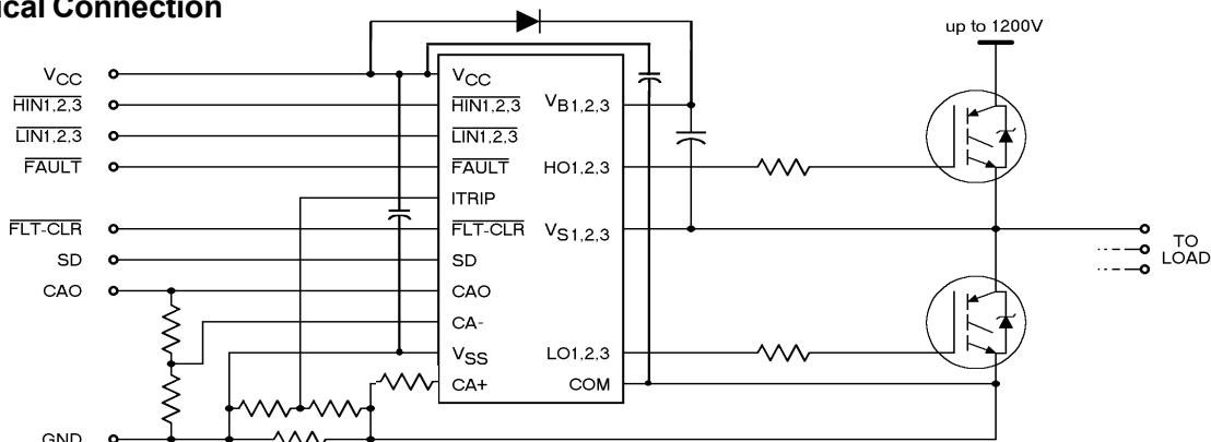
(Refer to Lead Assignments for correct pin configuration). This/These diagram(s) show electrical connections only.
