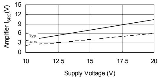
**Figure 50. Amplifier Output Source Current vs. Supply Voltage**
