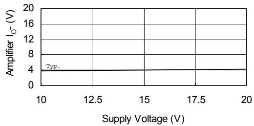
**Figure 53. Amplifier Output Low Short Circuit Current vs. Supply Voltage**
