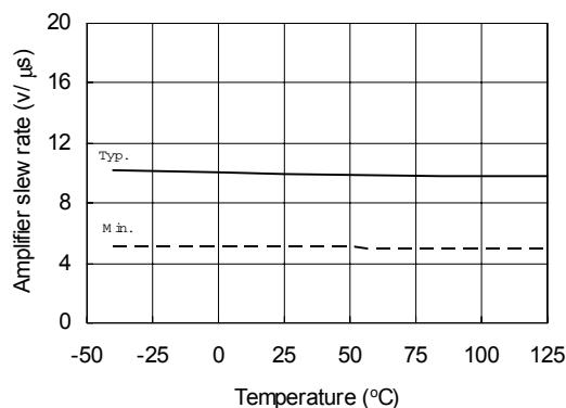
Figure 15A. Amplifier slew rate (+)
