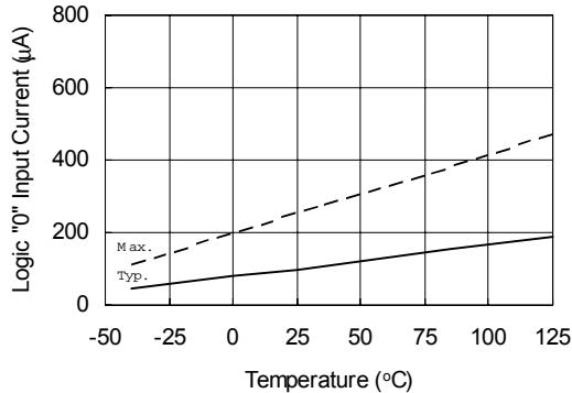
Figure 31A. Logic "0" Input Bias Current vs. Temperature
