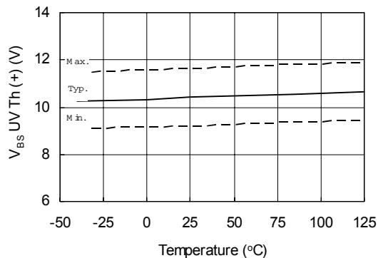
Figure 38A. IR2135/IR2235  $V_{BS}$  Undervoltage Threshold (+) vs. Temperature
