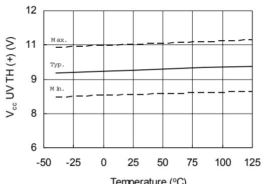
Figure 41A. IR2135/IR2235  $V_{cc}$  Undervoltage Threshold (-) vs. Temperature
