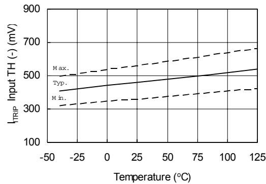
Figure 24A. I<sub>TRIP</sub> Input TH(-) vs. Temperature
