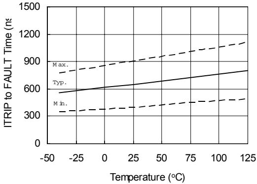
Figure 11A. ITRIP to FAULT Time
