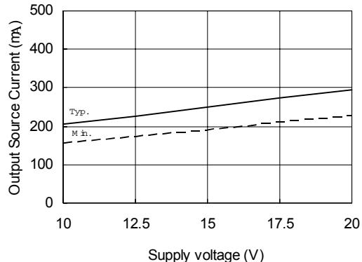
Figure 43B. Output Source Current vs. Supply Voltage
