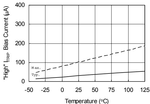
Figure 34A. "High"  $I_{TRIP}$  Bias Current vs. Temperature
