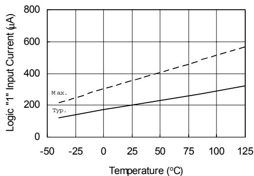
Figure 30A. Logic "1" Input Bias Current vs. Temperature
