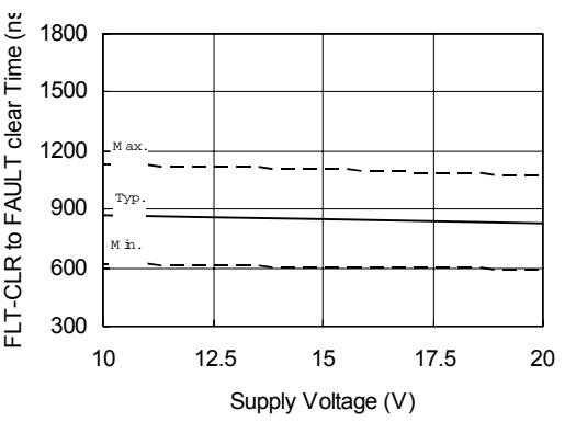
Figure 13B. FLT-CLR to FAULT clear Time
