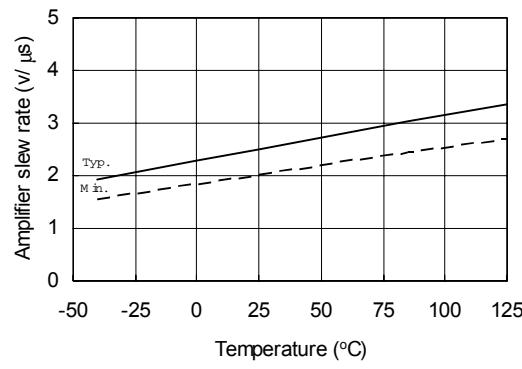
Figure 16A. Amplifier slew rate (-)
