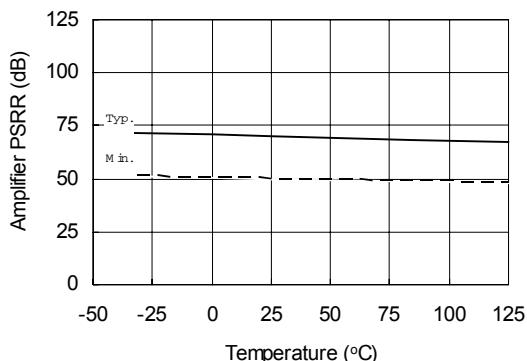
**Figure 47A. Amplifier Power Supply Rejection Ratio vs. Temperature**
