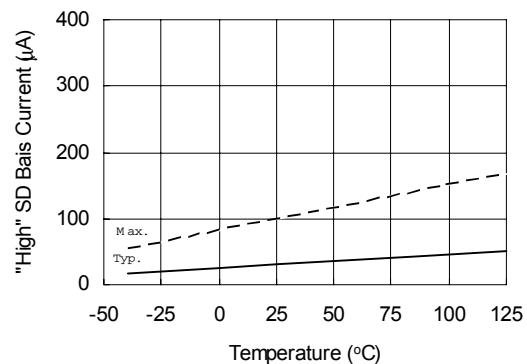
Figure 32A. "High" Shutdown Bias Current vs. Temperature
