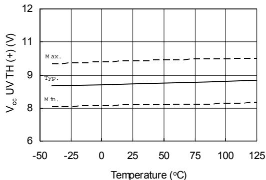
Figure 40B. IR2133/IR2233  $V_{cc}$  Undervoltage Threshold (+) vs. Temperature
