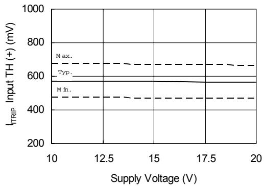
Figure 23B. I<sub>TRIP</sub> Input TH(+) vs. Voltage
