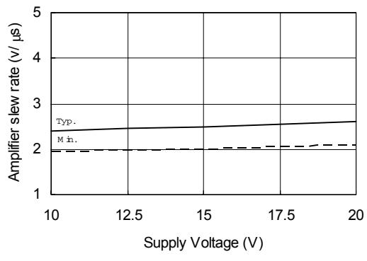
Figure 16B. Amplifier slew rate (-)
