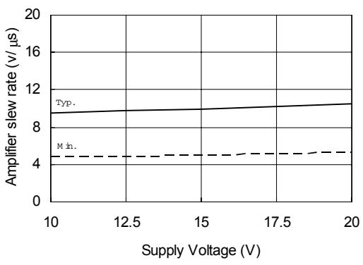
Figure 15B. Amplifier slew rate (+)
