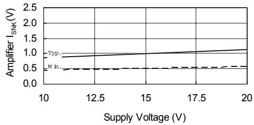
**Figure 51. Amplifier Output Sink Current vs. Supply Voltage**
