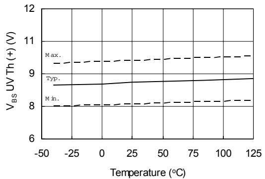
Figure 38B. IR2133/IR2233  $V_{BS}$  Undervoltage Threshold (+) vs. Temperature
