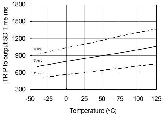
Figure 12A. ITRIP to output shutdown Time
