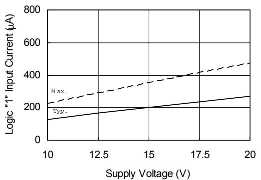
Figure 30B. Logic "1" Input Bias Current vs. Voltage
