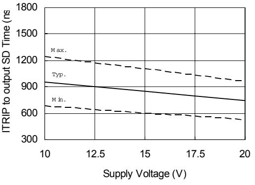
Figure 12B. ITRIP to output shutdown Time
