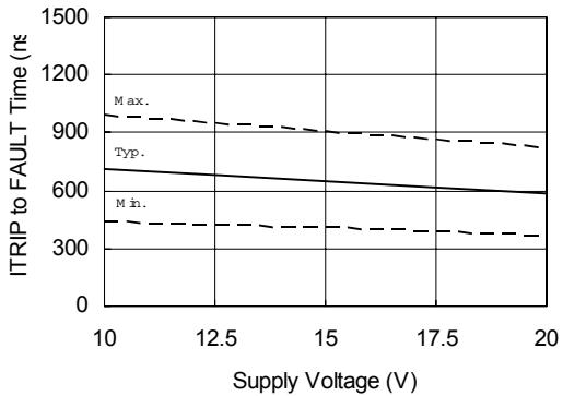
Figure 11B. ITRIP to FAULT Time
