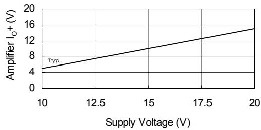
**Figure 52. Amplifier Output High Short Circuit Current vs. Supply Voltage**
