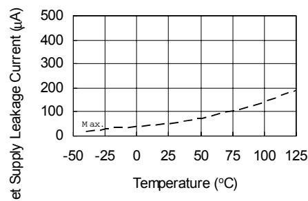
Figure 27A. Offset Supply Leakage Current vs. Temperature
