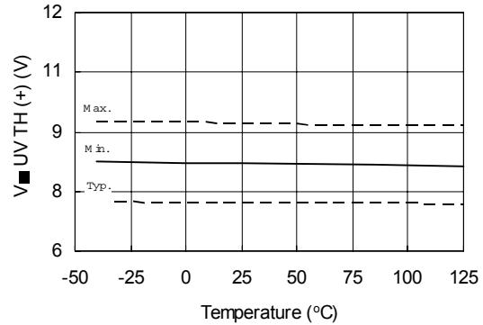
Figure 39B. IR2133/IR2233  $V_{BS}$  Undervoltage Threshold (-) vs. Temperature
