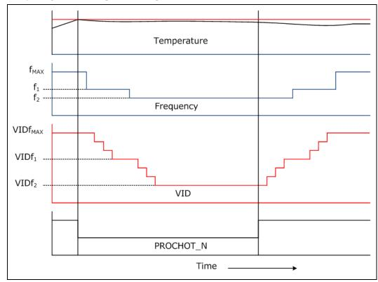
Figure 5-6. Frequency and Voltage Ordering
