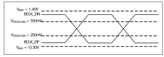
Figure 7-11. BCLK{0/1} Single Ended Clock Measurement Points for Delta Cross Point
