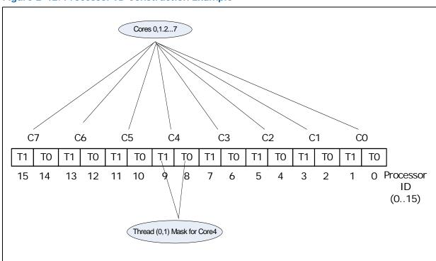
Figure 2-42. Processor ID Construction Example
