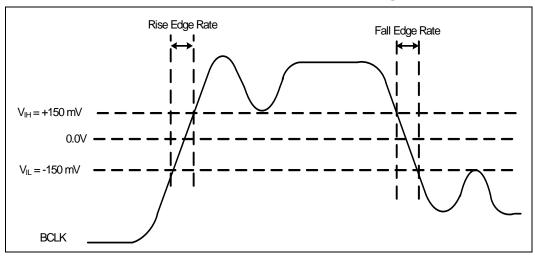
Figure 7-9. BCLK{0/1} Differential Clock Measurement Point for Ringback
