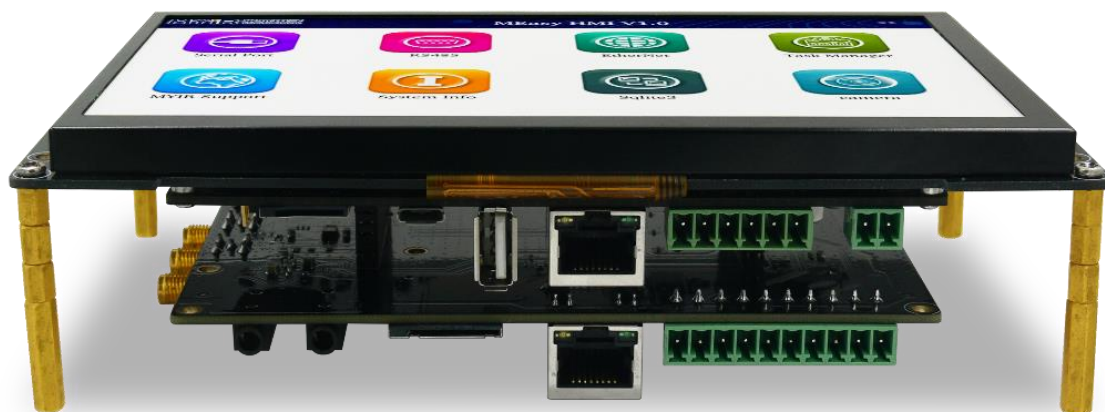
Figure 1-6 MYD-Y6ULX-CHMI Display Panel + MYB-Y6ULX-HMI-4GEXP IO Board
