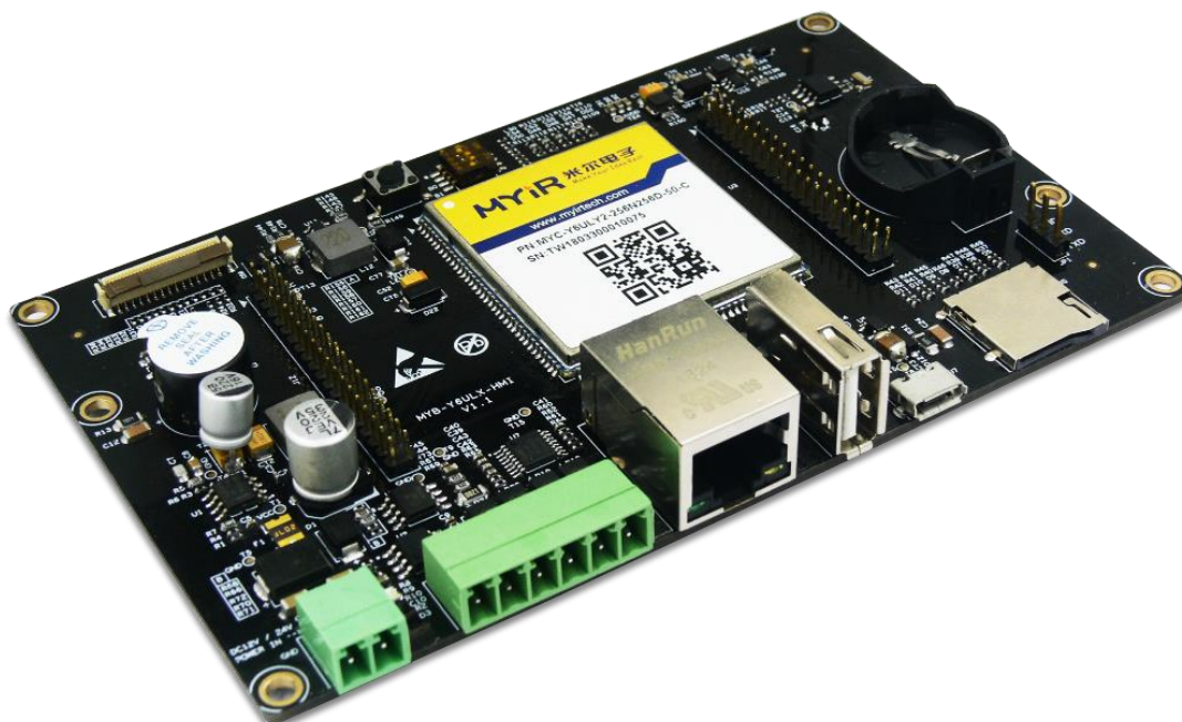
Figure 1-1 MYD-Y6ULX-HMI Development Board
