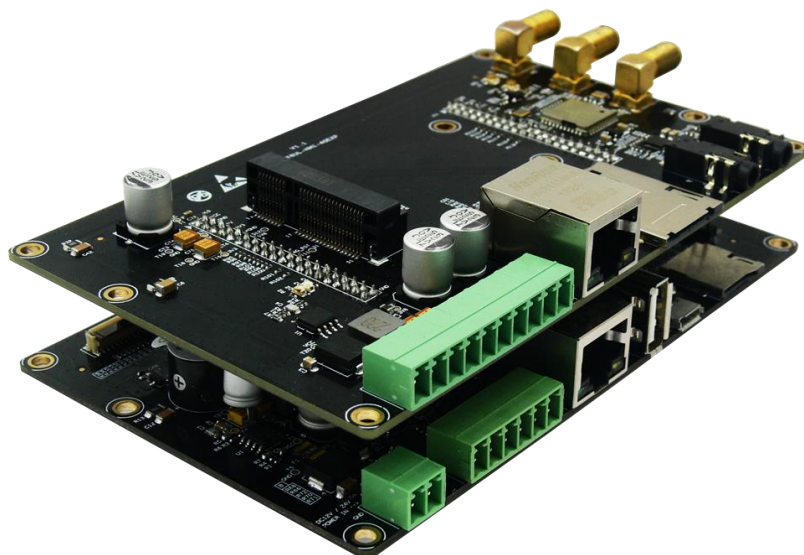
Figure 1-4 MYB-Y6ULX-HMI-4GEXP IO Board Mounted on MYD-Y6ULX-HMI
