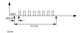
Fig. 18 - Ambient Light Measurement with Averaging = 8; using Continuous Conversion Mode
