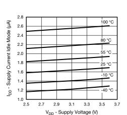
Fig. 2 - Idle Current vs. V<sub>DD</sub>
