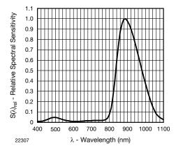
Fig. 7 - Relative Spectral Sensitivity vs. Wavelength (Proximity Sensor)
