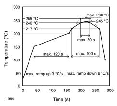
Fig. 19 - Lead (Pb)-free Reflow Solder Profile according to J-STD-020
