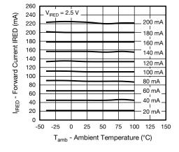
Fig. 4 - Forward Current vs. Temperature
