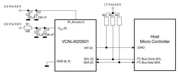
Fig. 12 - Application Circuit (x) = Pin Number
