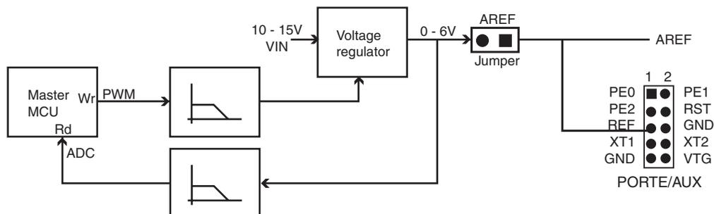
The AVR Studio-controlled analog reference voltage can also be used as an input to the analog comparator or for ADC measurements on the AVR. AVR's AREF signal can then be connected to VTG.
