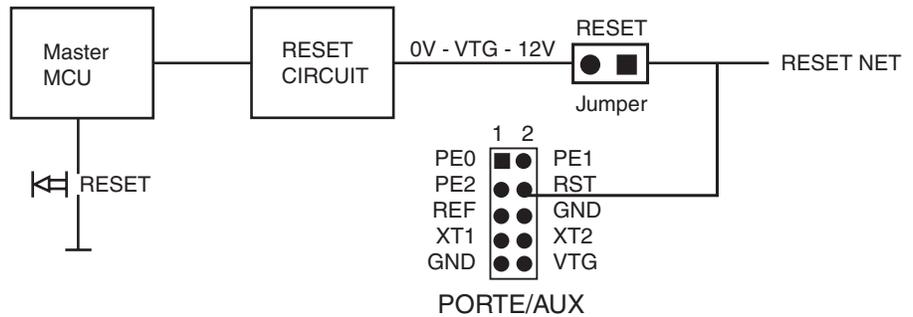
**Note:** During High-voltage Programming, STK500 applies 12V to the AVR's RESET line. Thus, an external reset circuit not capable of handling this must be disconnected before High-voltage Programming the AVR.
