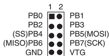
**Figure 3-12.** PORTB SPI Pinout (28-pin Analog Parts)
