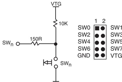
**Note:** In the AVR, the user can enable internal pull-ups on the input pins, removing the need for an external pull-up on the push-button. In the STK500 design, we have added an external 10K pull-up to give all users a logical “1” on SWn when the push-button is not pressed. The 150R resistor limits the current going into the AVR.
