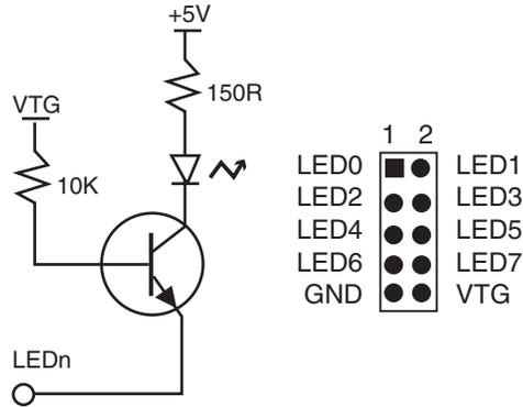
**Note:** The AVR can source or sink enough current to drive a LED directly. In the STK500 design, a transistor with two resistors is used to give the same amount of light from the LED, whatever the target voltage (VTG) may be and to turn off the LEDs when VTG is missing.
