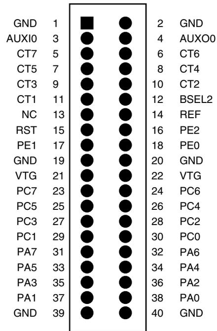
**Figure 3-35.** Expansion Connector 1 Pinout
