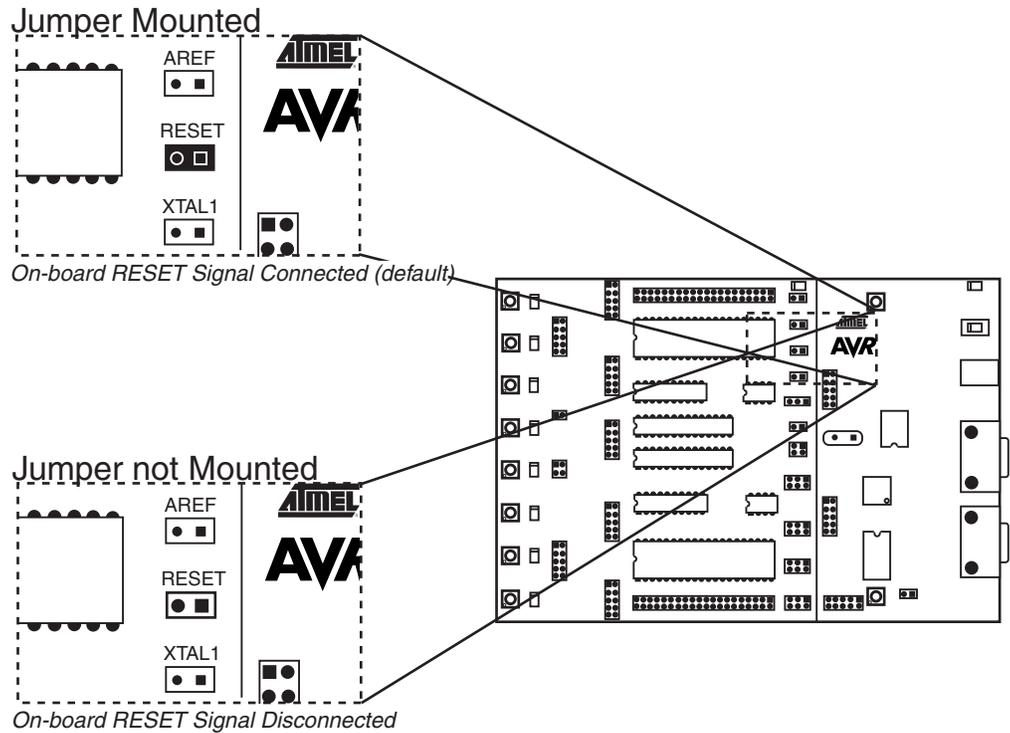
The STK500 master microcontroller controls the RESET signal to the target AVR. The RESET signal is accessible on the PORTE/AUX header; this pin can also be used for external RESET signal. Figure 3-26 shows the internal connection of the RESET signal.
