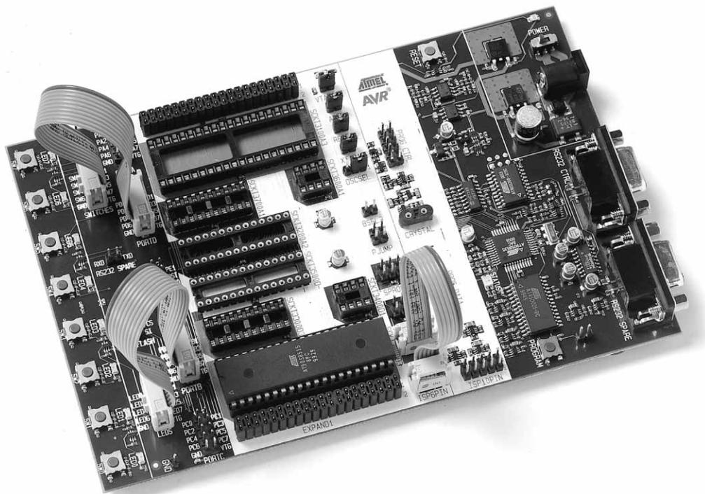
The starter kit can be configured for various clock and power sources. A complete description of the jumper settings is explained in paragraph 3.8 on page 3-15 and on the reverse side of the starter kit.
