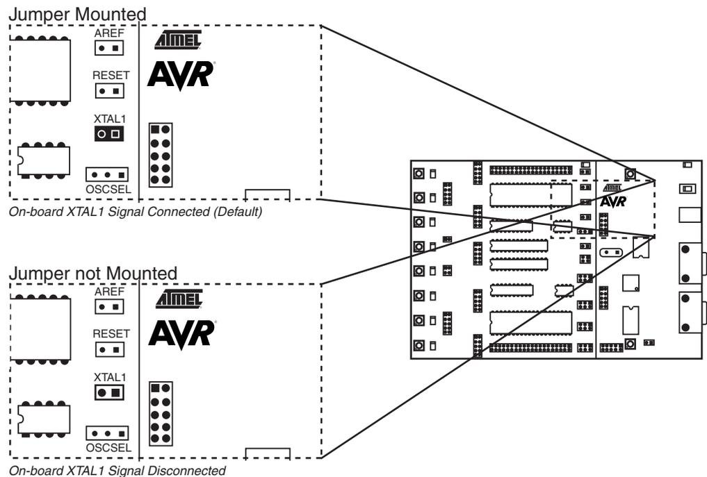
When the XTAL1 jumper is not mounted, an external clock source or crystal can be connected to the PORTE header. This is shown in Figure 3-30.
