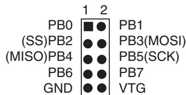
**Figure 3-13.** Connection of I/O Pins to DataFlash for AT90S8515
