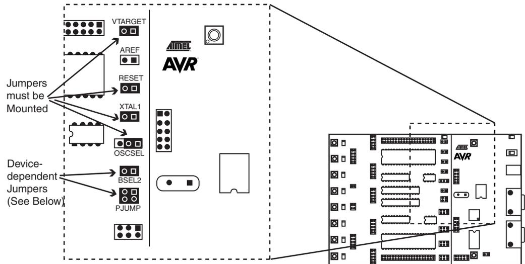
Hardware setup for parallel High-voltage Programming:
