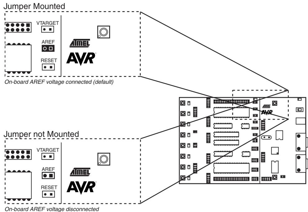
The STK500 master microcontroller controls the analog reference voltage using the internal PWM. The AVR's AREF signal is also accessible on the PORTE header; this pin can also be used for external AREF signal. Figure 3-24 shows the internal connection of the AREF signal.
