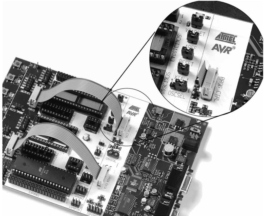
Some of the jumper settings on STK500 must be changed when using High-voltage Programming. Figure 3-18 explains these jumper settings.
