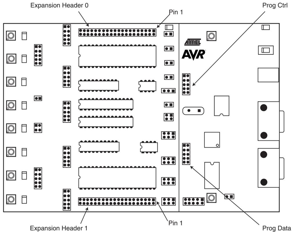
**Figure 3-34.** Expansion Connector 0 Pinout
