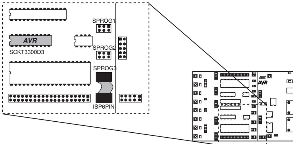
It is not necessary to remove the 6-wire cable from its ISP position while running a program in the AVR. The port pins used for ISP programming can be used for other purposes in your program.
