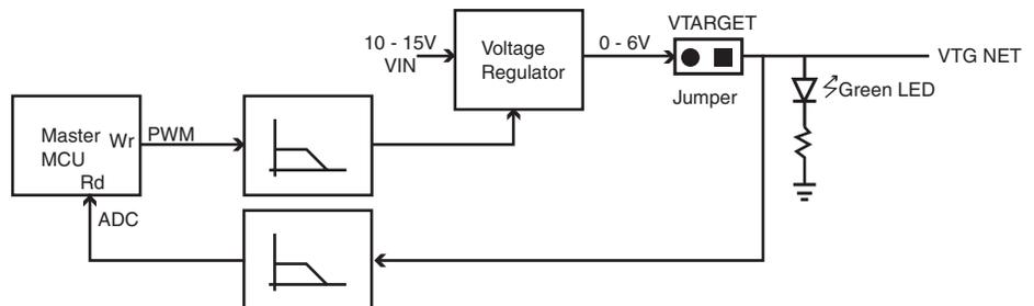
**Note:** The green LED will light when there is a voltage available on the VTG NET. It's impossible to use the debug or programming area of STK500 without VTG.
