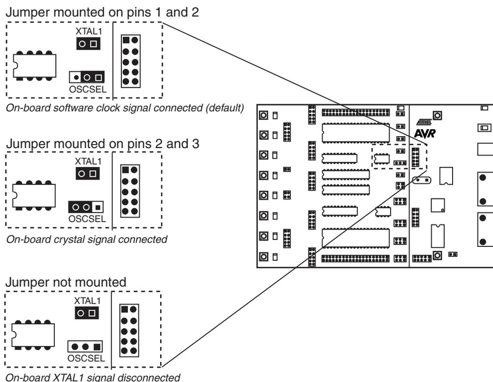
When programming AVR in High-voltage Programming mode, OSCSEL should be mounted on pins 1 and 2 to give the master microcontroller control of the target clock. This is explained in detail in Section 3.7.2 on page 3-11.
