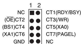
The Prog Ctrl signals are normally used for the control signals when parallel High-voltage Programming an AVR device.
