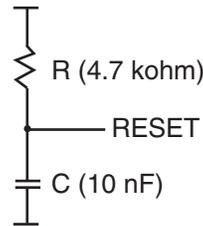
If the external pull-up resistor is too low (<4.7 kΩ), STK500 will not be able to pull the RESET line low.
