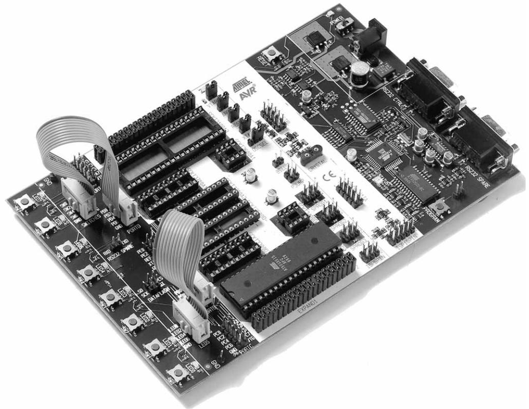
Any I/O port of the AVR can be connected to the LEDs and switches using the 10-wire cables. The headers are supplied with VTG (target  $V_{CC}$ ) and GND lines in addition to the signal lines.
