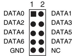
The Prog Data signals are used for the data bus when parallel High-voltage Programming an AVR device. During ISP programming, DATA5 is used as MOSI, DATA6 is used as MISO, and DATA7 is used for SCK.
