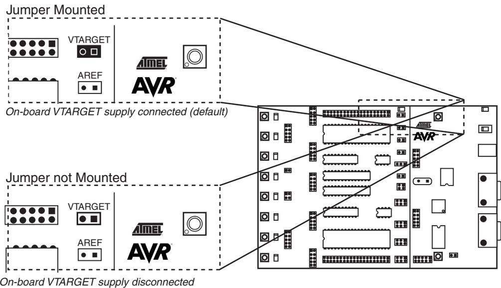
The STK500 master microcontroller controls the target voltage using the internal PWM. Figure 3-22 shows the internal connection of the VTARGET signal.
