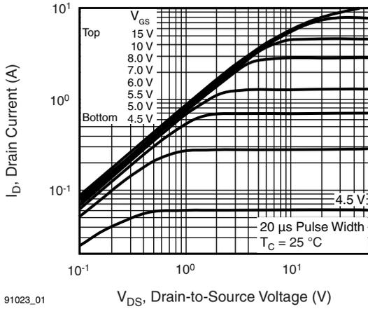
Fig. 1 - Typical Output Characteristics,  $T_C = 25\text{ }^\circ\text{C}$
