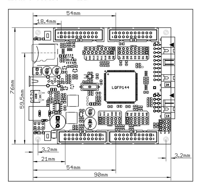
The three highest elements on the board in order from the tallest to the shortest are: capacitor C46 - 17.2 mm (0.677") over the pcb; USB host connectors -14.3 mm (0.563"); capacitators C11 and C3 - 11.5 mm (0.453").
