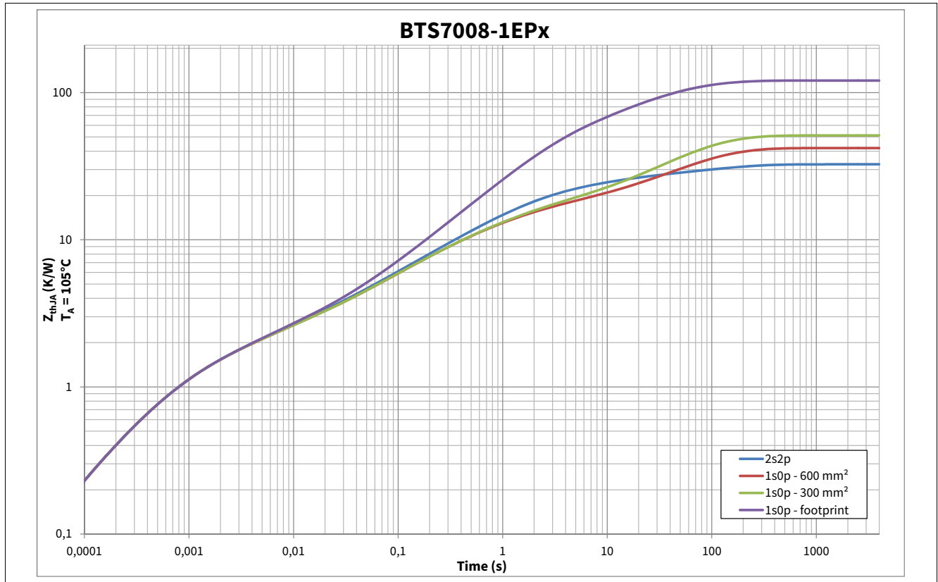
Figure 9 Typical Thermal Impedance. PCB setup according Chapter 4.4.1
