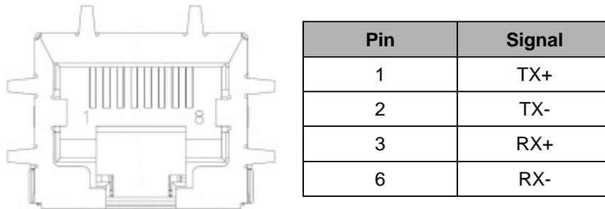
Figure 21. RJ-45 PIN Assignment
