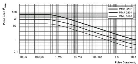
Maximum pulse load, single pulse; applicable if  $\bar{P} \rightarrow 0$  and  $n \le 1000$  and  $\hat{U} \le \hat{U}_{max}$ ; for permissible resistance change equivalent to 8000 h operation
