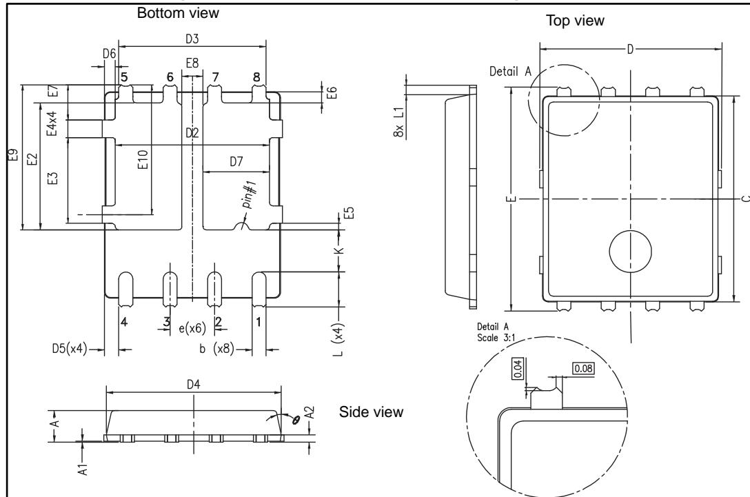
Table 6: PowerFLAT™ 5x6 dual pad package mechanical data
