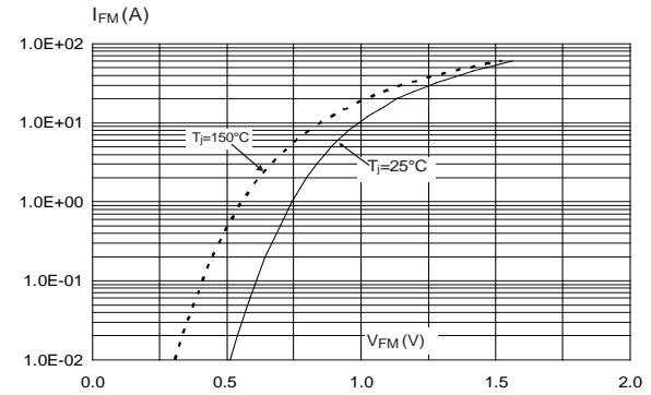
**Figure 3: Forward voltage drop versus forward current (maximum values, per diode)**
