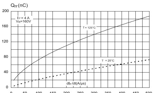
**Figure 6: Reverse recovery time versus dI<sub>F</sub> / dt (typical values, per diode)**
