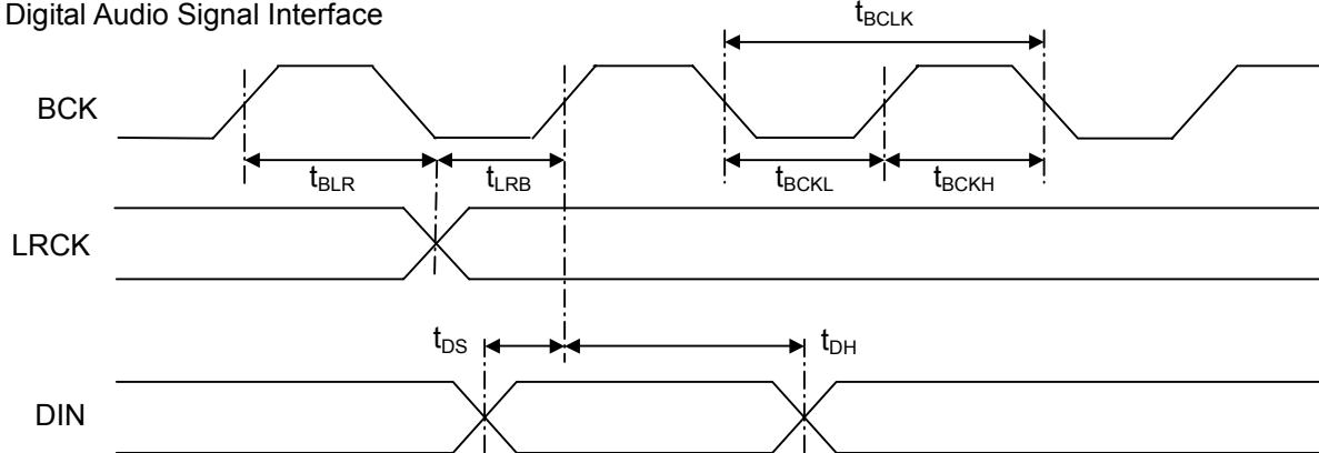
( $T_a=25^\circ\text{C}$ ,  $V_{DD}=V_{DDL}=V_{DDR}=3.3\text{V}$ , unless otherwise noted)
