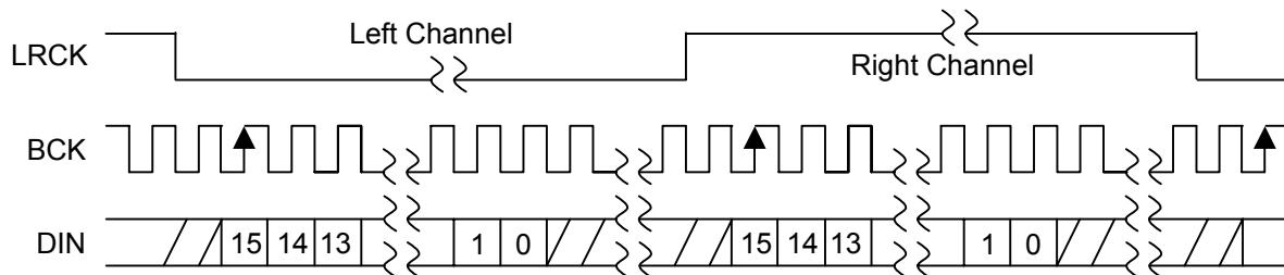
Figure 3.1. 16 bits I<sup>2</sup>S Data Format
