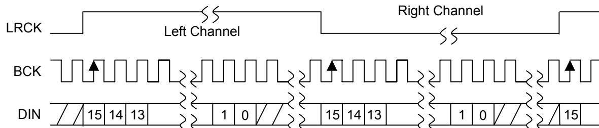
Figure 3.2. 16 bits MSB Justified Data Format
