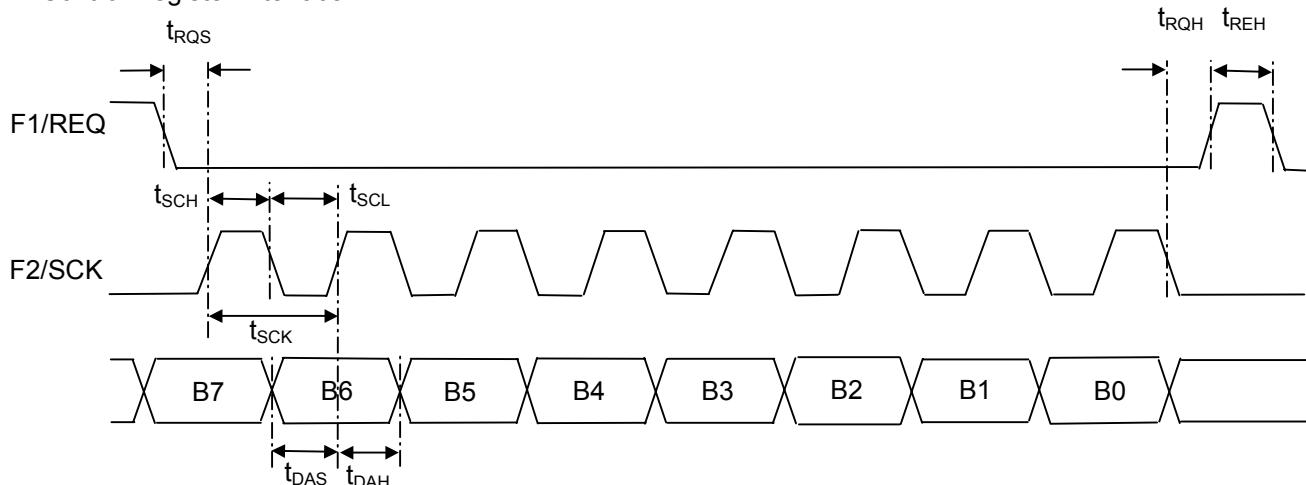
( $T_a=25^\circ\text{C}$ ,  $V_{DD}=V_{DDL}=V_{DDR}=3.3\text{V}$ , unless otherwise noted)
