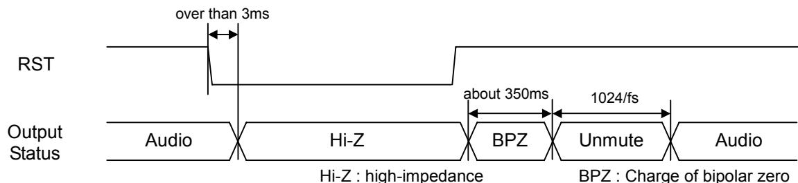
Figure 1. Reset Timing
