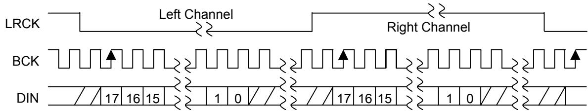
Figure 3.4. 18 bits I<sup>2</sup>S Data Format
