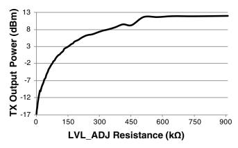
Figure 5: NT Series Transceiver Output Power vs. LVL\_ADJ Resistance
