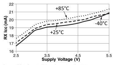
Figure 10: NT Series Transceiver RX Current Consumption vs. Supply Voltage
