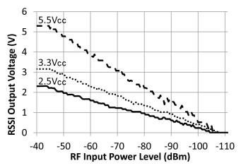
Figure 11: NT Series Transceiver RSSI Voltage vs. Input Power
