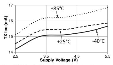
Figure 9: NT Series Transceiver TX Current Consumption vs. Supply Voltage at OdBm
