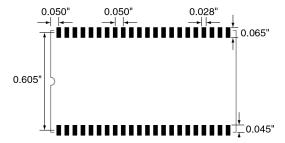
Figure 31: Recommended PCB Layout
