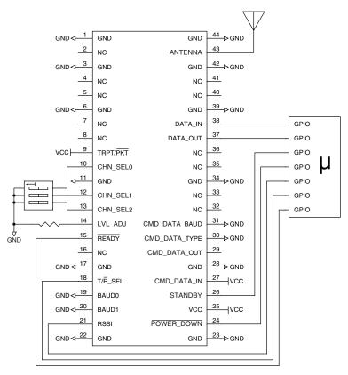
Figure 26: NT Transceiver Typical Application
