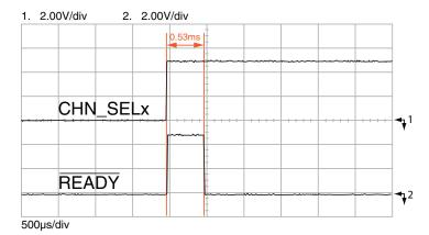
Figure 18: NT Series Transceiver Channel Change Time
