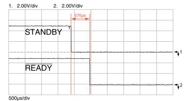
Figure 14: NT Series Transceiver Turn-On Time from Standby
