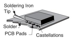
Figure 32: Soldering Technique
