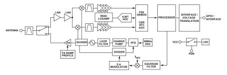
Figure 20: NT Series Transceiver Block Diagram
