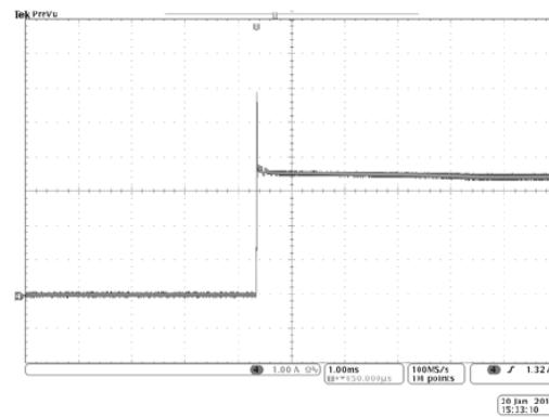
Fig. 13:  $V_{IN}=1.8V$ ,  $V_{REF}=0.9V$  sink short circuit
