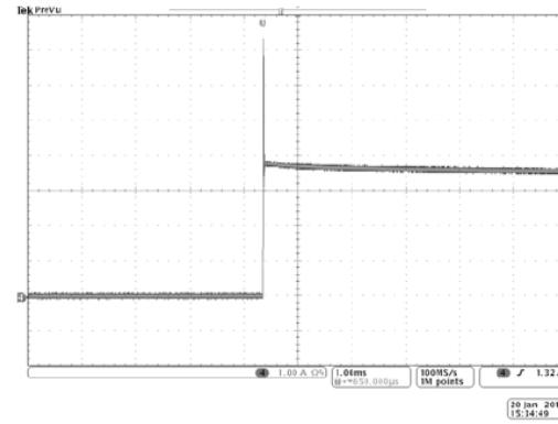
Fig. 14:  $V_{IN}=2.5V$ ,  $V_{REF}=1.25V$  sink short circuit
