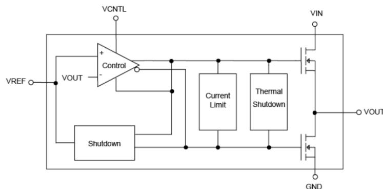
Fig. 2: XRP2997 Block Diagram
