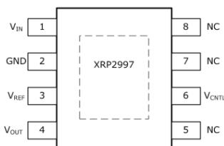
Fig. 3: XRP2997 Pin Assignment
