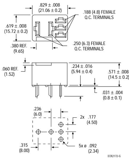
Wiring harness, bracket mount socket
