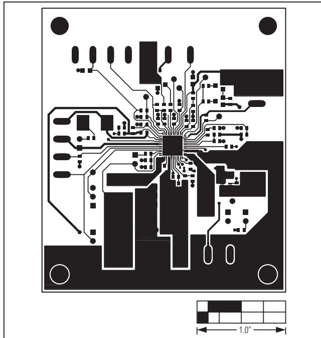
*Figure 3. MAX17114 EV Kit PCB Layout—Component Side*
