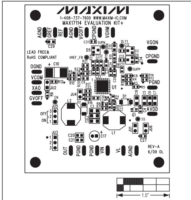
*Figure 2. MAX17114 EV Kit Component Placement Guide—Component Side*
