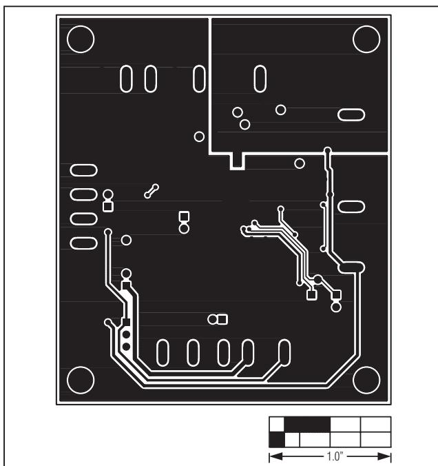
Figure 4. MAX17114 EV Kit PCB Layout—Solder Side
