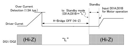
**CAUTION:**Over Current Detection circuits is only intended to provide temporary protection against irregular conditions such as an output short-circuit; they do not necessarily guarantee the complete IC safety. Therefore, output short-circuit(short to VCC or GND) the ground fault Since the IC may be destroyed, the design of routing output line, VCC, and GND lines sufficient attention Please.
