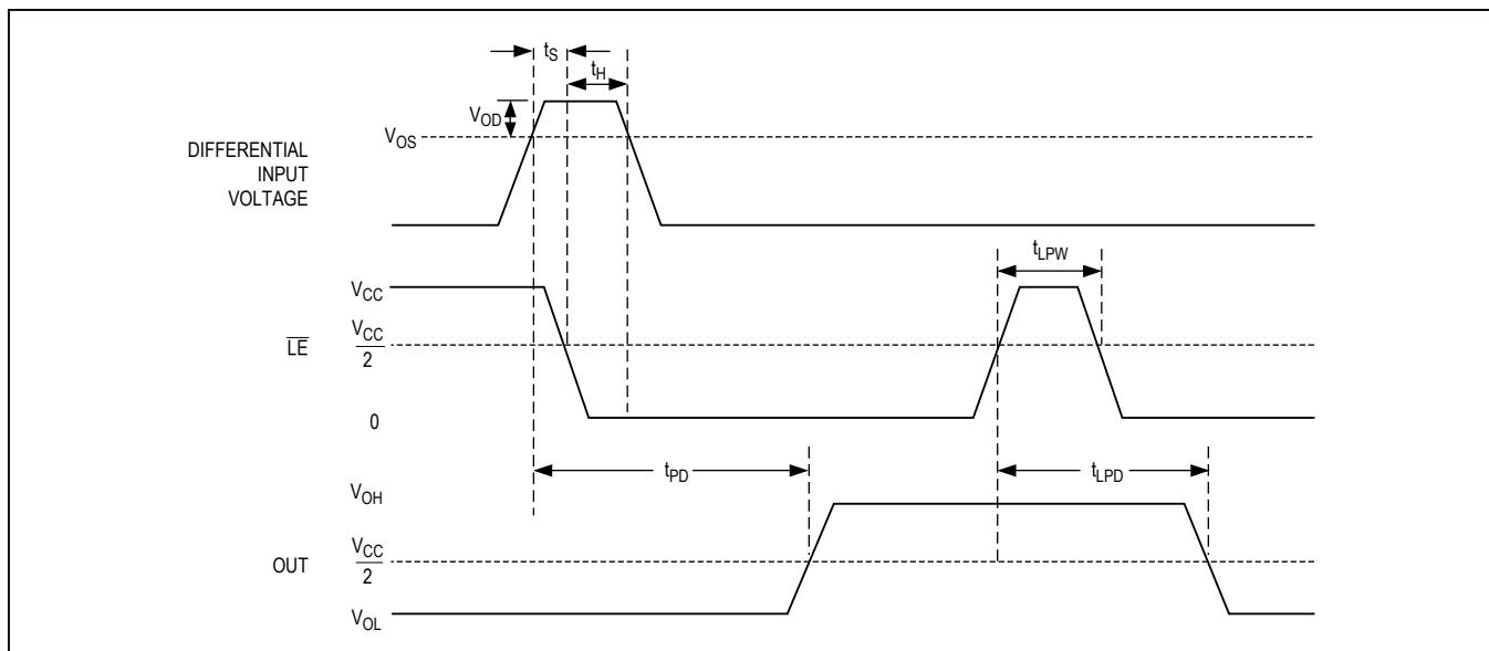
Figure 2. MAX9141 Timing Diagram with Latch Operator
