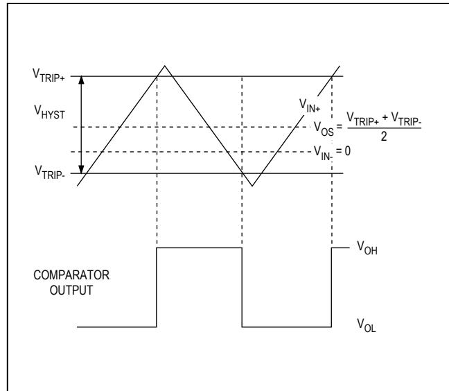
Figure 1. Input and Output Waveform, Noninverting Input Varied
