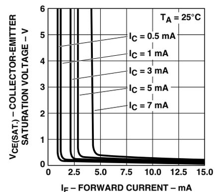
Figure 3. Collector-emitter saturation voltage vs. forward current.
