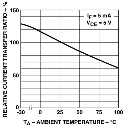
Figure 7. Relative current transfer ratio vs. temperature.
