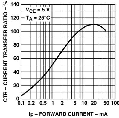
Figure 5. Current transfer ratio vs. forward current.
