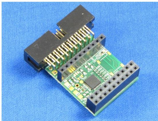
Figure 2.1 Top view of IQS316 EV-Kit controller board
