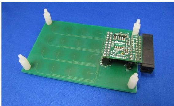
Figure 3.2 16-Key Touchpanel with controller board attached
