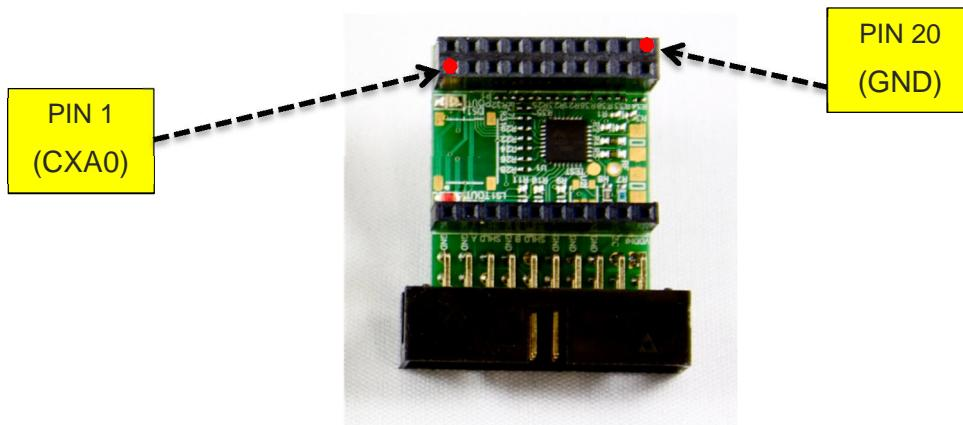
**Figure 6.2 IQS316 Controller Module**
