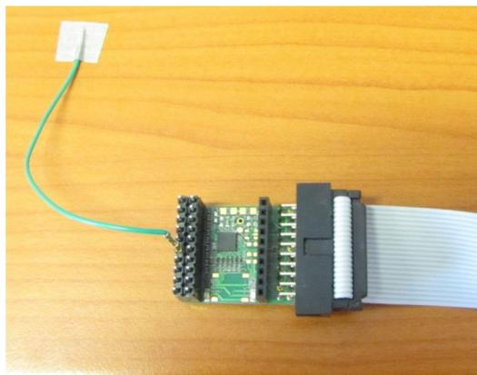
**Figure 6.3 Simple touchkey connected to IQS316 Controller**
