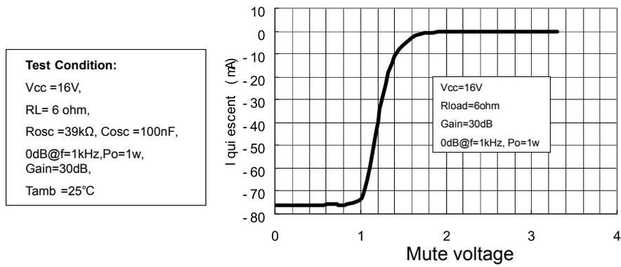
Figure 32. Current consumption vs. voltage on pin STBY
