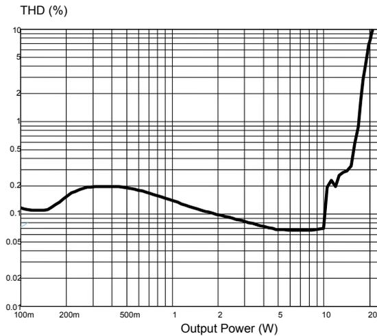
**Figure 36. THD vs. output power (100 Hz)**
