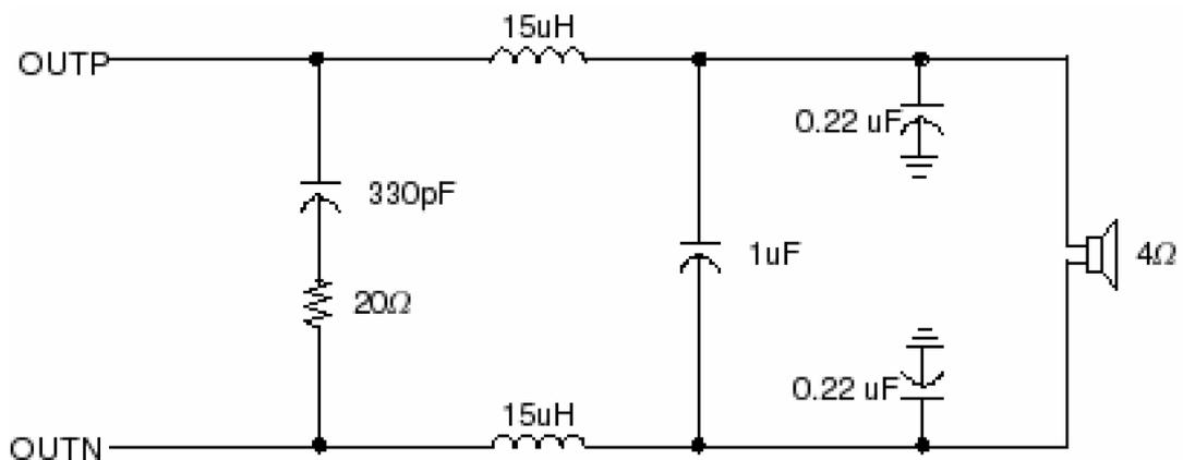
Figure 57. Typical LC filter for an 4 Ω speaker
