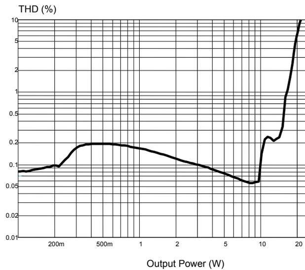
Figure 21. THD vs. output power (100 Hz)
