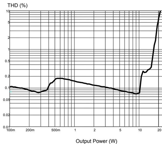
Figure 6. THD vs. output power (100 Hz)
