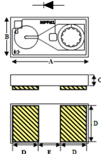
1. Backside metal: 0.1  $\mu$ m thick.
