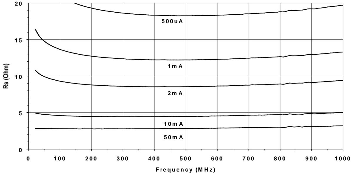
MA4SPS402 Rs vs I at 100 MHz and 1,000 MHz
