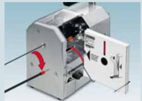
Stripping and crimping automatically
