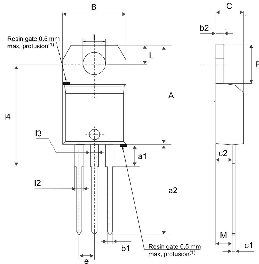
(1) Resin gate position accepted in one of the two positions or in the symmetrical opposites.
