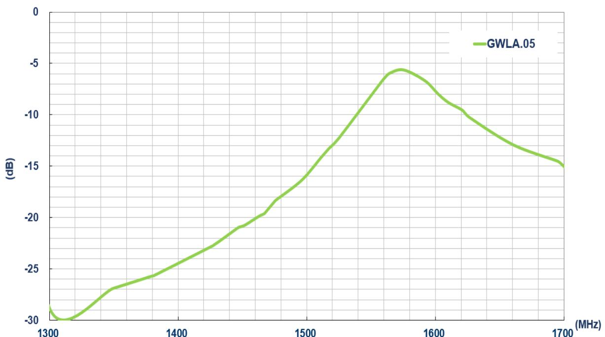
**Figure 6** GPS Average Gain(dB) on 30x15mm ground plane
