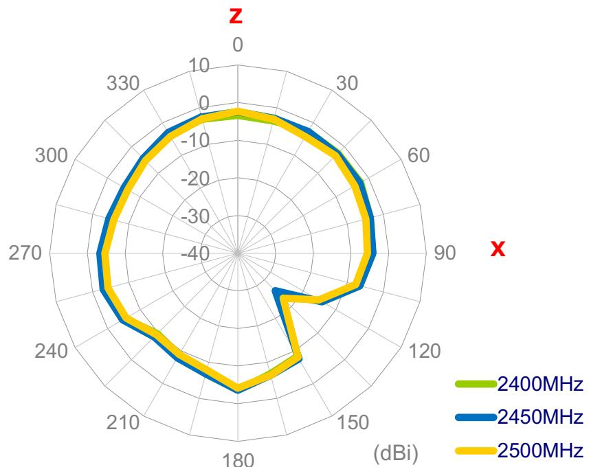
**Figure 26** X-Z polar plot of Wi-Fi on 80x40mm ground plane
