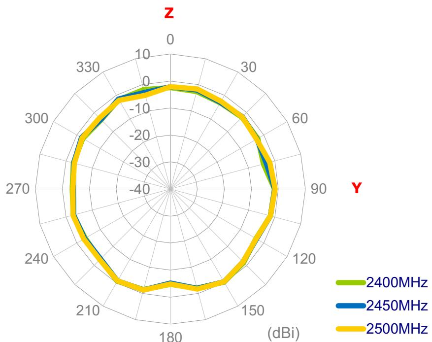
**Figure 30** Y-Z polar plot of Wi-Fi on 30x15mm ground plane
