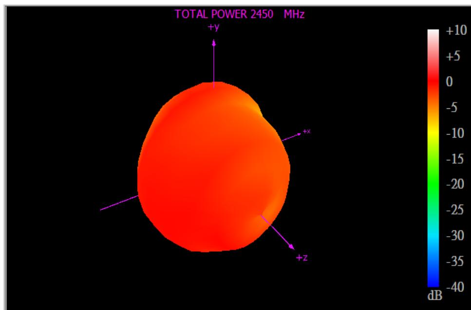
**Figure 34** Wi-Fi 3D radiation pattern 30x15mm ground plane
