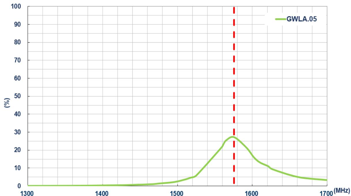
**Figure 4** GPS Efficiency(%) on 30x15mm ground plane
