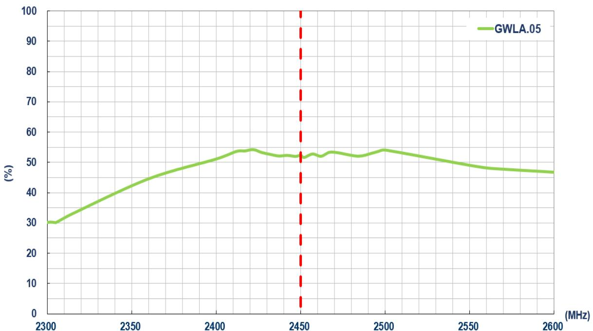
**Figure 12** Wi-Fi Efficiency(%) on 30x15mm ground plane
