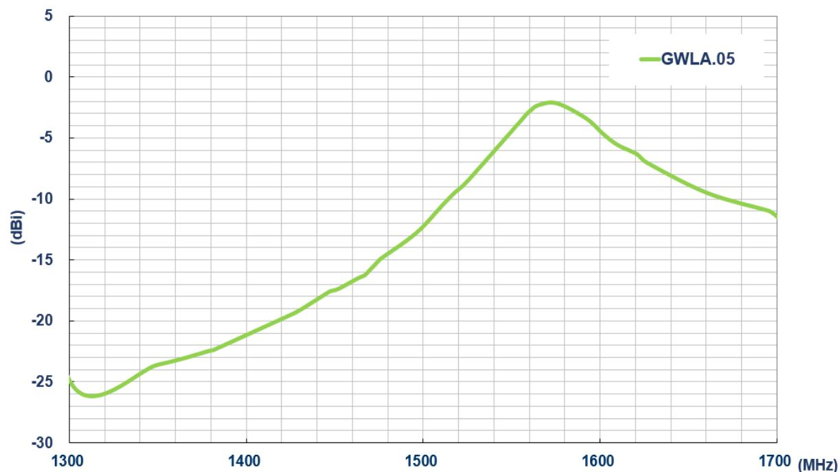
**Figure 8** GPS Peak Gain(dBi) on 30x15mm ground plane
