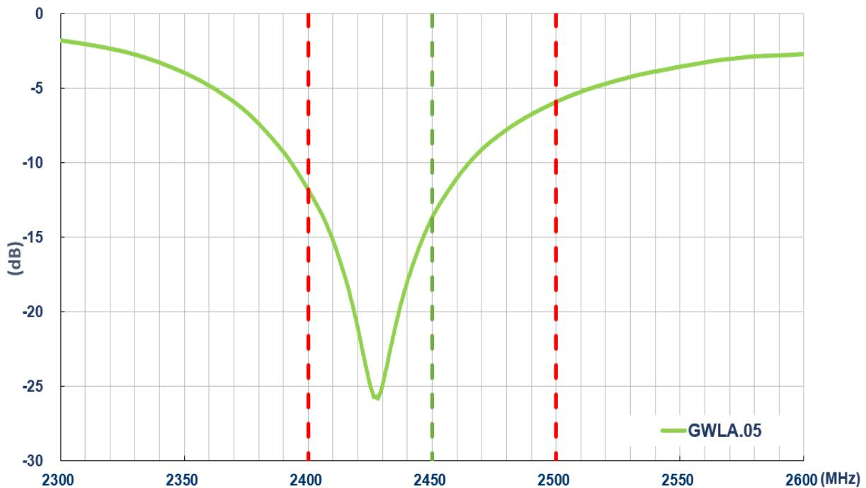
**Figure 9** Wi-Fi Return Loss on 80x40mm ground plane
