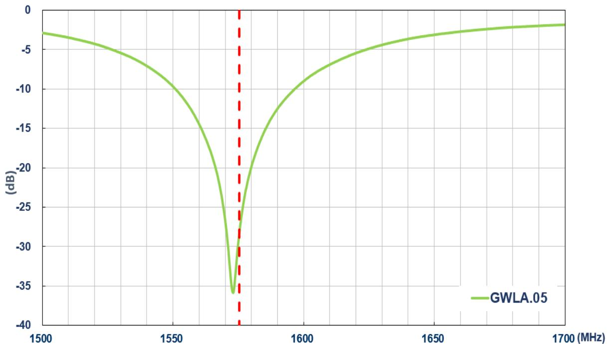
**Figure 1** GPS Return Loss(dB) on 80x40mm ground plane
