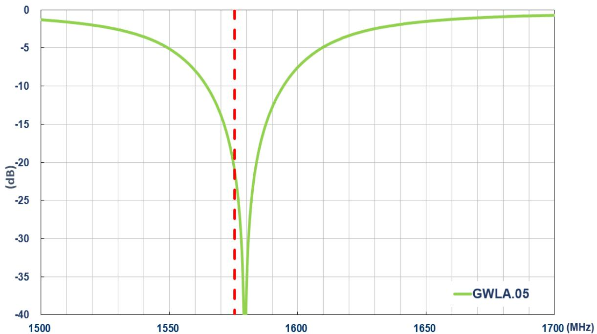
**Figure 2** GPS Return Loss(dB) on 30x15mm ground plane
