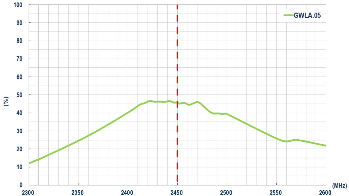
**Figure 11** Wi-Fi Efficiency(%) on 80x40mm ground plane
