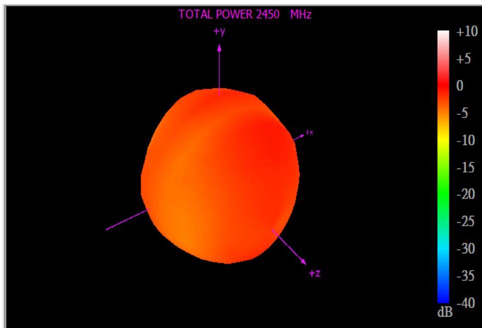
**Figure 33** Wi-Fi 3D radiation pattern 80x40mm ground plane
