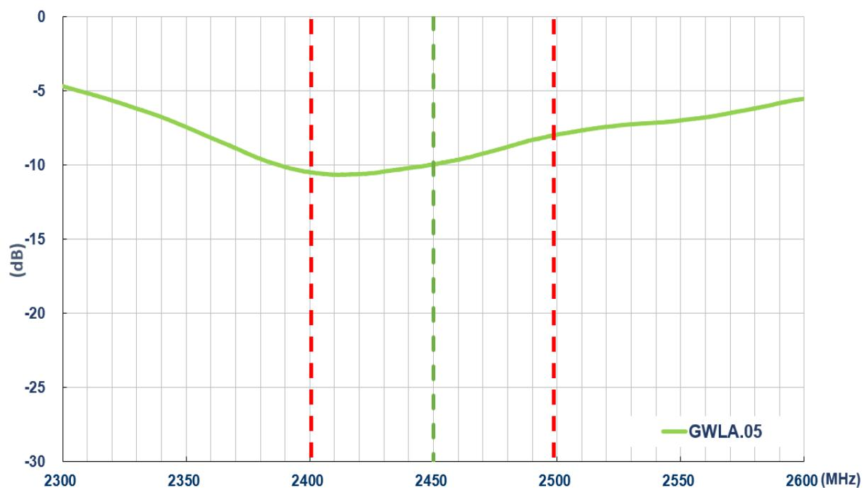
**Figure 10** Wi-Fi Return Loss(dB) on 30x15mm ground plane
