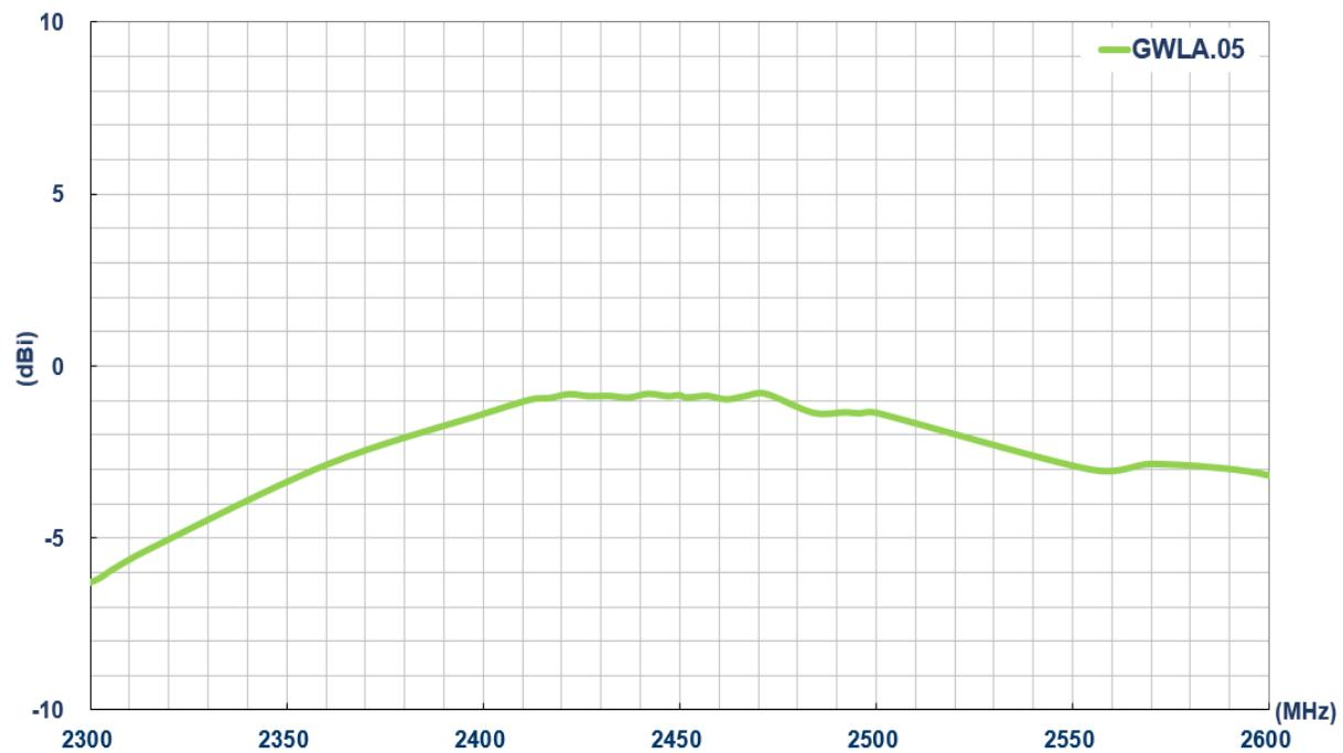
**Figure 15** Wi-Fi Peak Gain on 80x40mm ground plane
