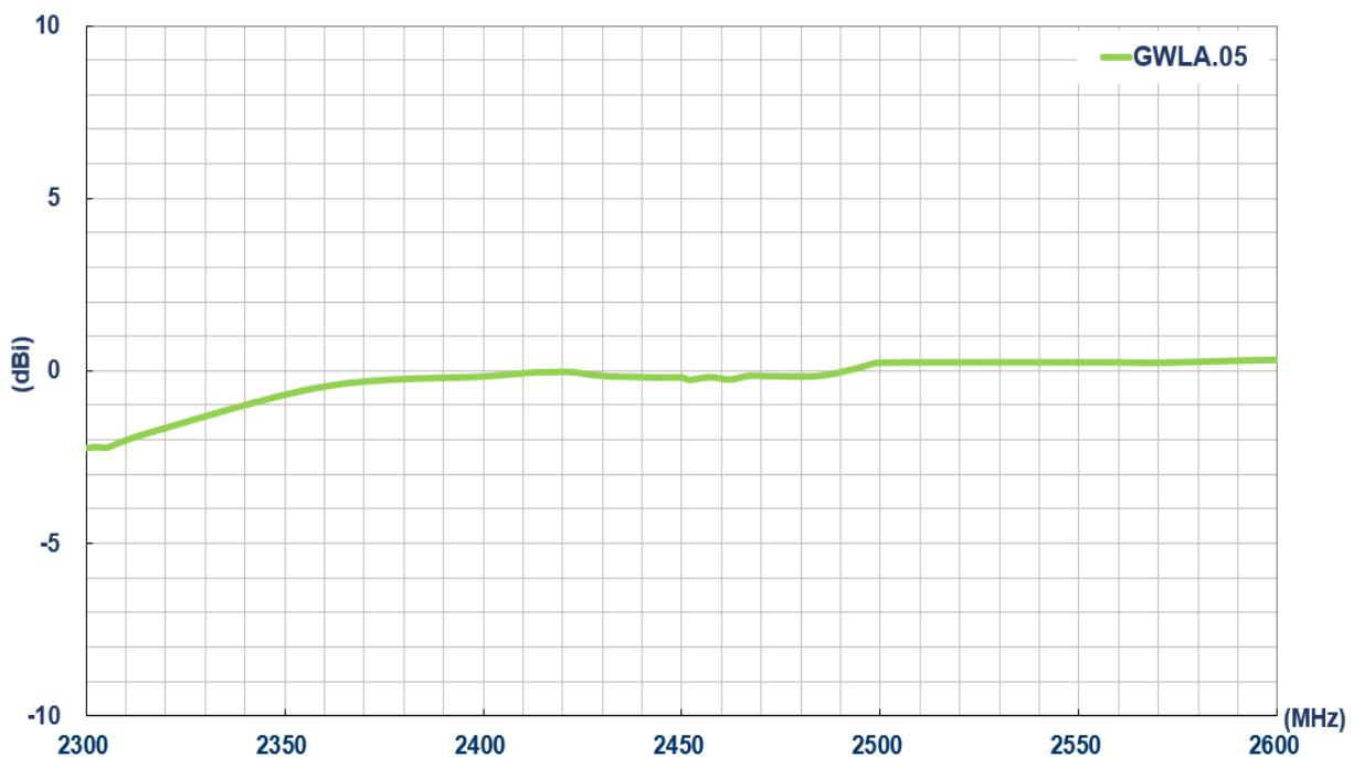
**Figure 16** Wi-Fi Peak Gain(dBi) on 30x15mm ground plane
