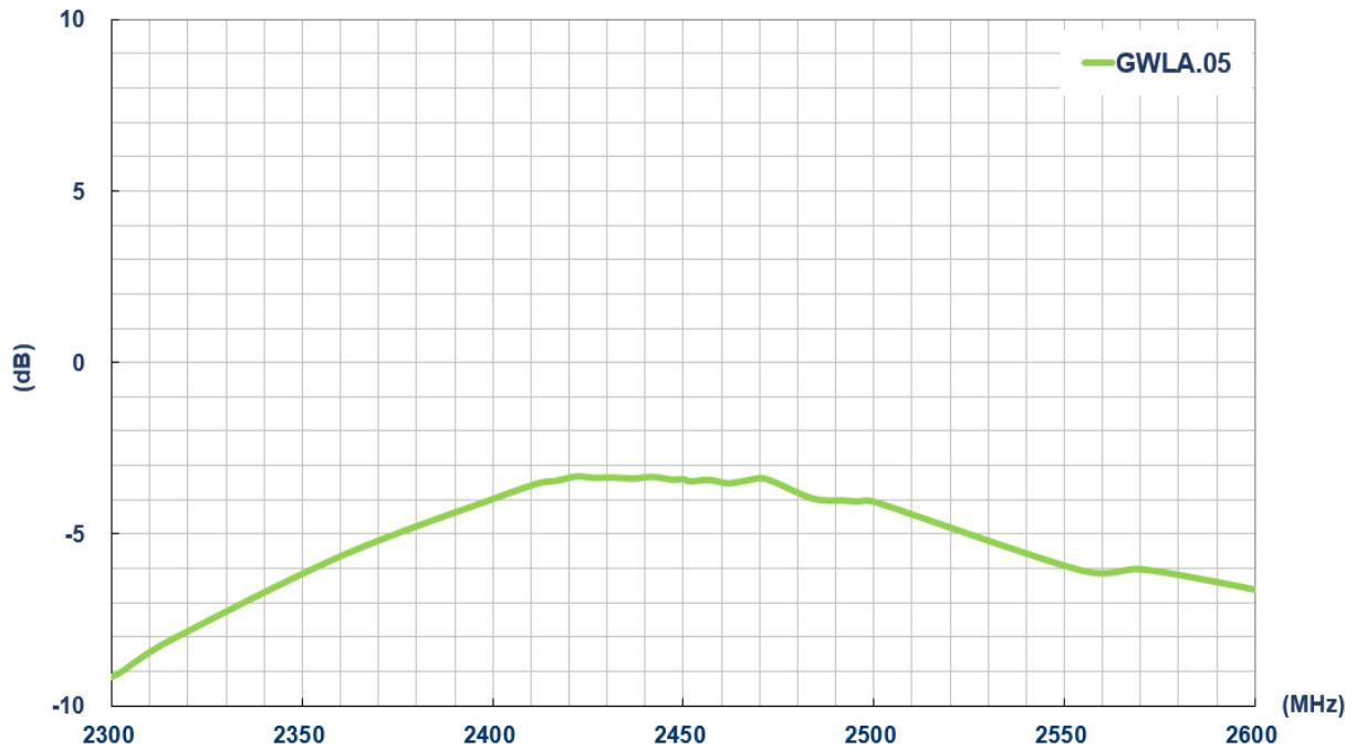
**Figure 13** Wi-Fi Average Gain(dB) on 80x40mm ground plane
