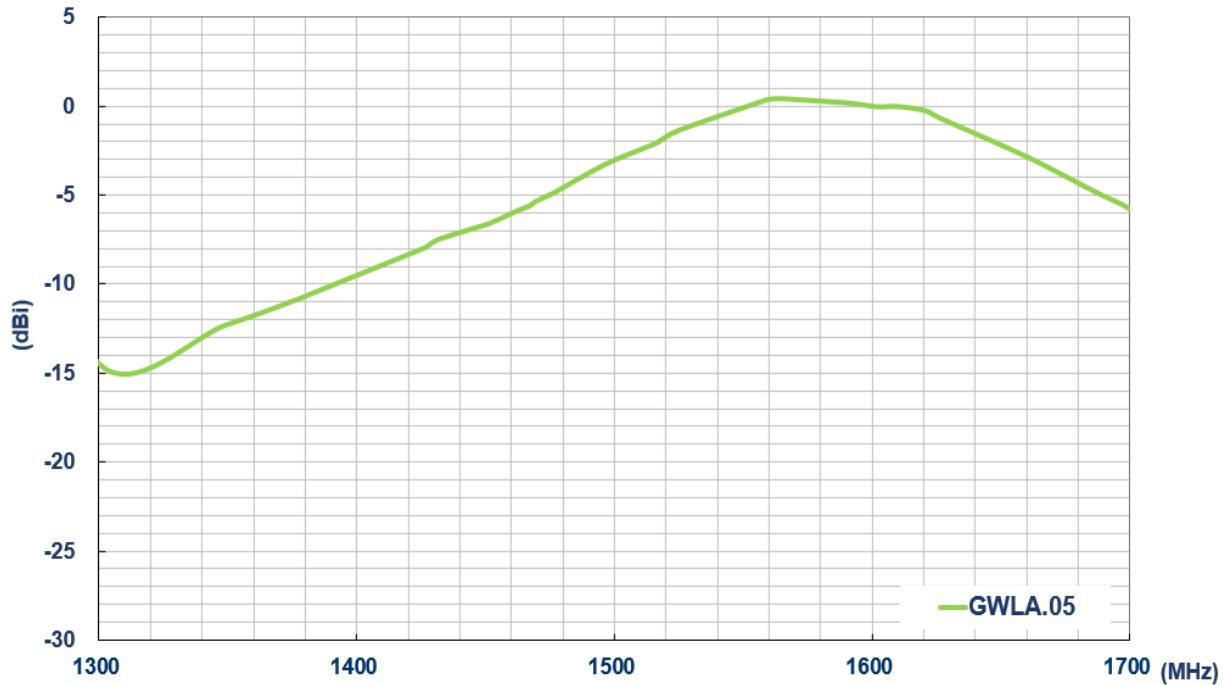
**Figure 7** GPS Peak Gain(dBi) on 80x40mm ground plane
