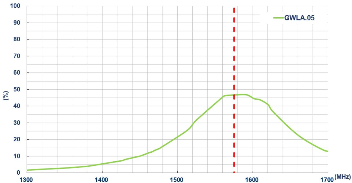
**Figure 3** GPS Efficiency(%) on 80x40mm ground plane
