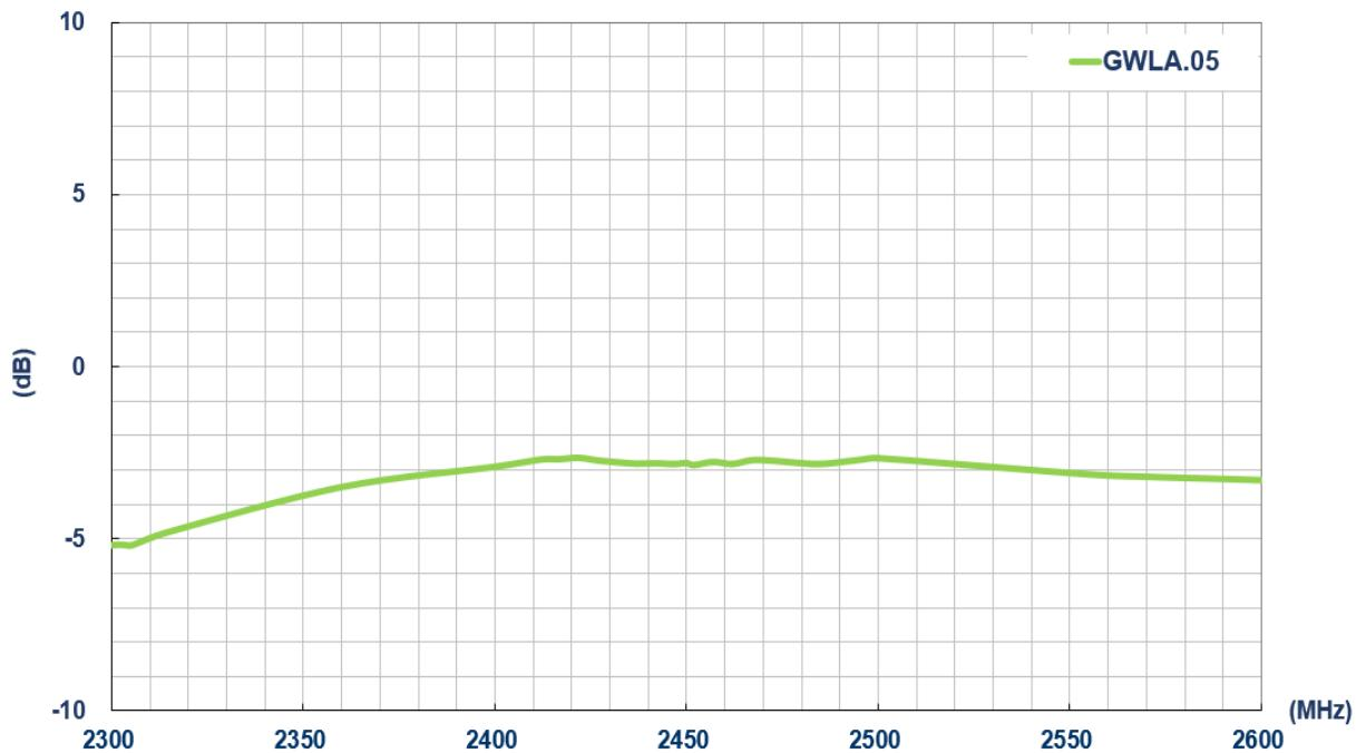
**Figure 14** Wi-Fi Average Gain(dB) on 30x15mm ground plane
