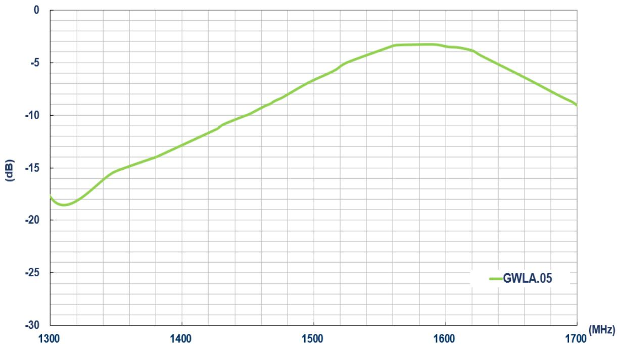
**Figure 5** GPS Average Gain(dB) on 80x40mm ground plane
