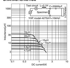
Test equipmentL: 4194A IMPEDANCE/GAIN-PHASE ANALYZER HP, or equivalent
