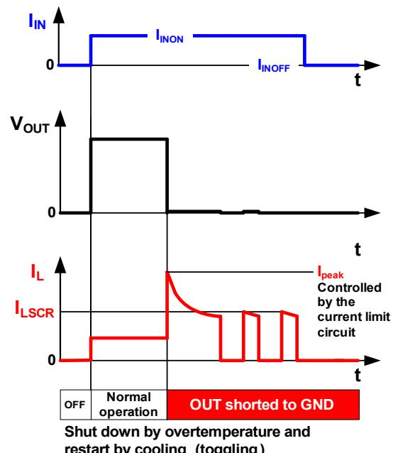
Figure 7 Protective behaviour waveforms of the ITS41k0S-ME-N
