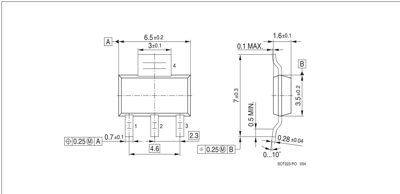
**Figure 8 PG-SOT223-4 (Plastic Dual Small Outline Package, RoHS-Compliant)**
