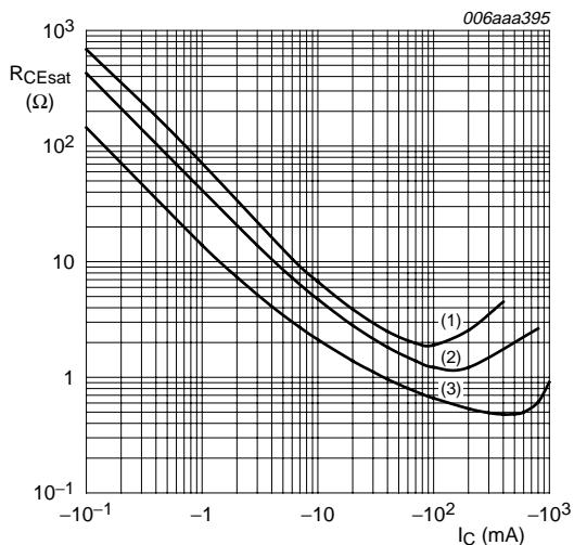
**Fig 8.** TR1 (PNP): Collector-emitter saturation resistance as a function of collector current; typical values
