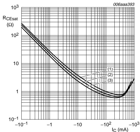
**Fig 7.** TR1 (PNP): Collector-emitter saturation resistance as a function of collector current; typical values
