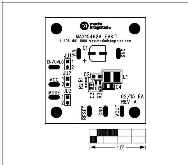
Figure 1. MAX15462A EV Kit Component Placement Guide—Component Side
