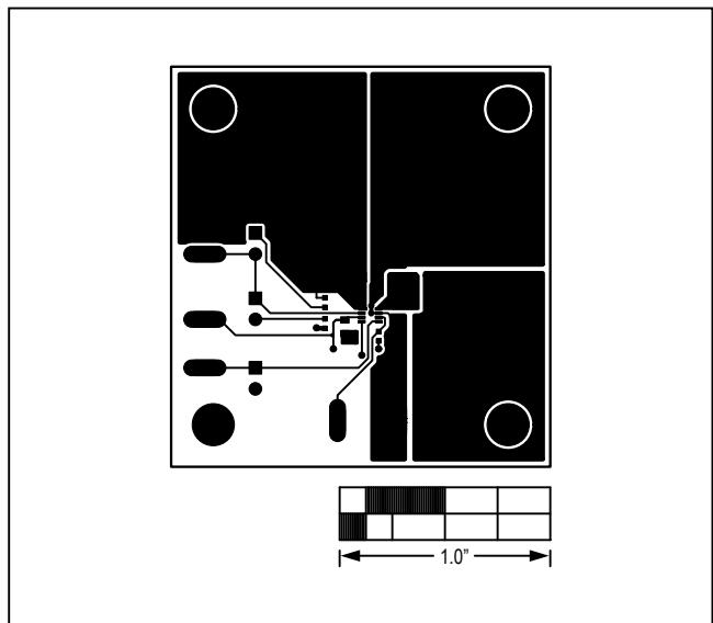
Figure 2. MAX15462A EV Kit PCB Layout—Component Side
