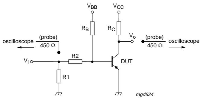
$I_C = -1$  A;  $I_{Bon} = -50$  mA;  $I_{Boff} = 50$  mA;  $R_1 =$  open;  $R_2 = 45$   $\Omega$ ;  $R_B = 145$   $\Omega$ ;  $R_C = 10$   $\Omega$
