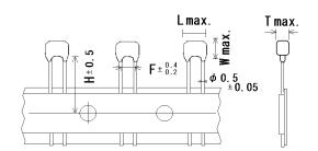
Inside Crimp Taping (Lead Code: M2)
