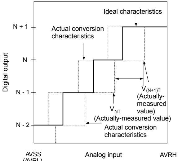
$$\text{Integral Nonlinearity of digital output } N = \frac{V_{NT} - \{1 \text{ LSB} \times (N-1) + V_{ZT}\}}{1 \text{ LSB}} \quad [\text{LSB}]$$
