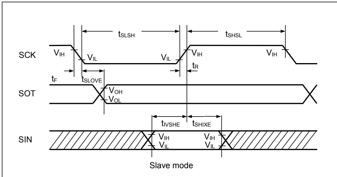
**(5-1-2) Normal Synchronous Transfer (SCR:SPI = 0) and Serial Clock Output Signal Detect Level "L"
