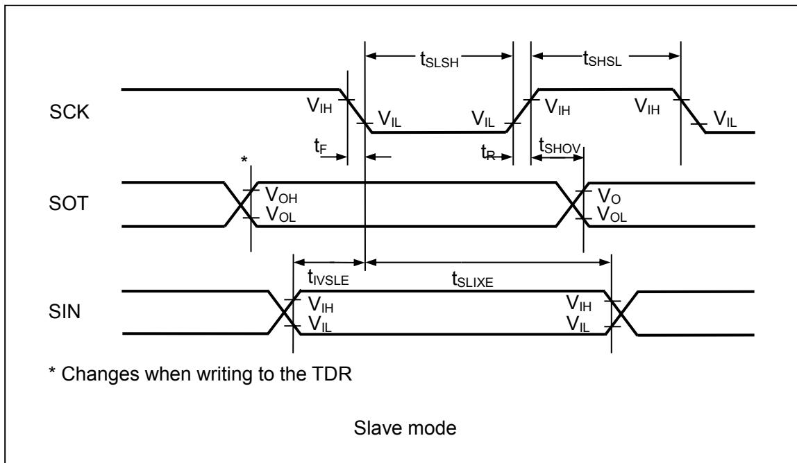
**(5-1-4) SPI Supported (SCR:SPI = 1), and Serial Clock Output Signal Detect Level "L" (SMR:SCINV = 1)**
