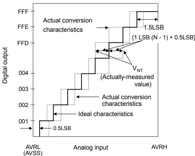
$$\text{Total error of digital output } N = \frac{V_{NT} - \{1 \text{ LSB} \times (N-1) + 0.5\text{LSB}\}}{1\text{LSB}} \text{ [LSB]}$$
