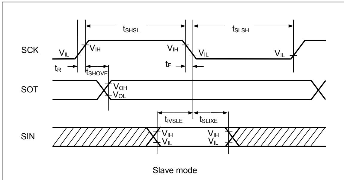
**(5-1-3) SPI Supported (SCR:SPI = 1), and Serial Clock Output Signal Detect Level "H" (SMR:SCINV = 0)**
