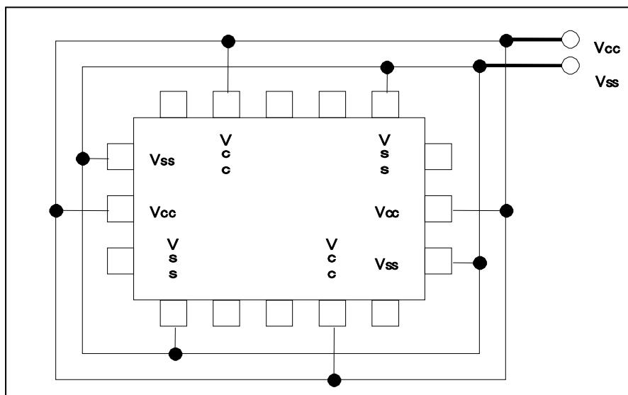
In addition, consider connecting with low impedance from the power supply source to the V<sub>CC</sub> and V<sub>SS</sub> of this device.
