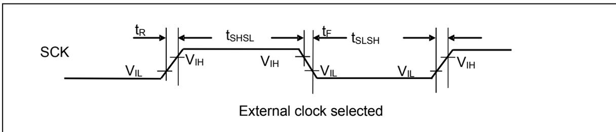
10.4.7.3 *LIN Interface (v2.1) (LIN Communication Control Interface (v2.1)) Timing (SMR:MD[2:0] = 011B)*
