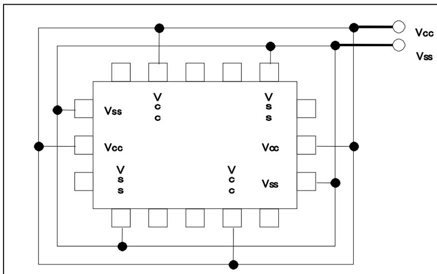
In addition, consider connecting with low impedance from the power supply source to the  $V_{CC}$  and  $V_{SS}$  of this device.
