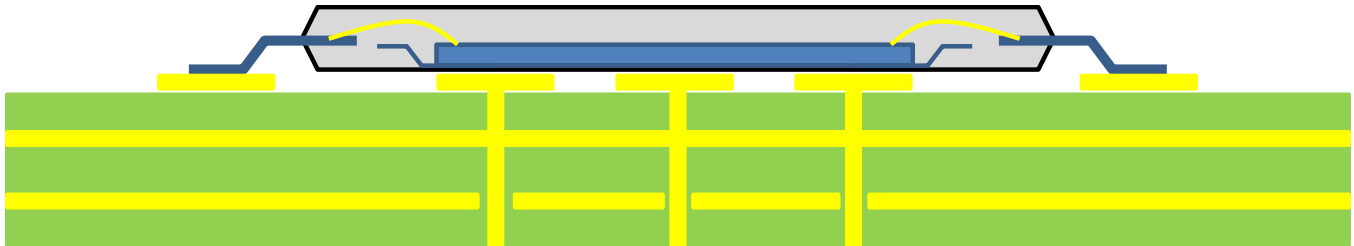
Figure10.2-1: Example thermal via holes on PCB.
