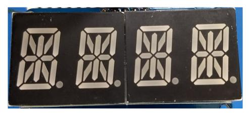
To access the individual digits, it's the same as with the 7-segment display. However, the 14-segment display can take any alphanumeric character. For example:
