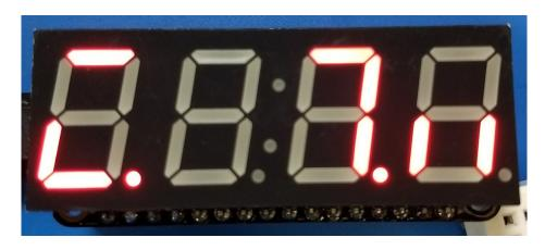
The above command will create the 7-segment class using the default I2C address of the display (0x70). If you've changed the I2C address (like when using multiple backpacks or displays) you can override it in the initializer using an optional **address** keyword argument.
