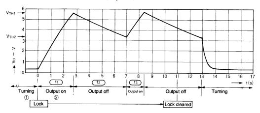
Automatic recovery circuit pin C voltage
