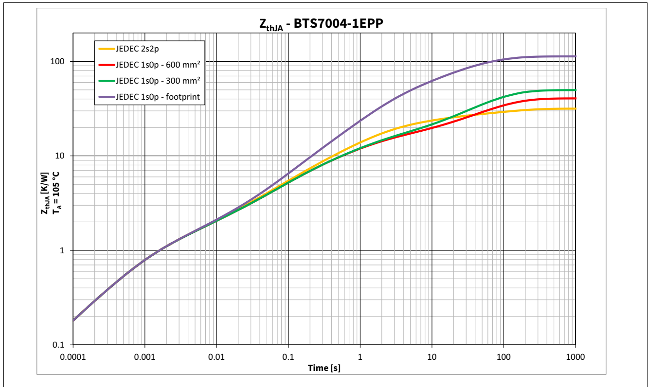
Figure 9 Typical Thermal Impedance. PCB setup according Chapter 4.4.1
