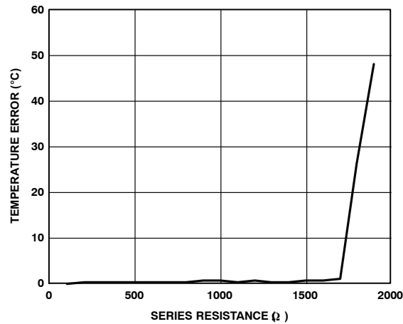
Figure 13. Temperature Error vs. Series Resistance
