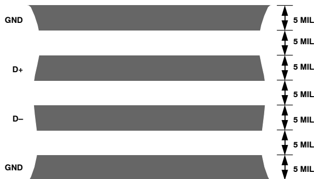
Figure 22. Typical Arrangement of Signal Tracks
