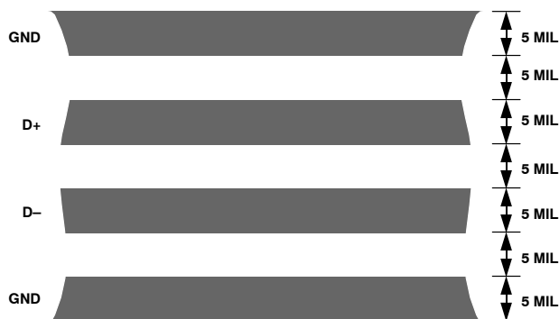
Figure 22. Typical Arrangement of Signal Tracks
