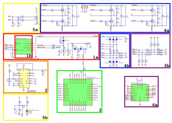
Figure 3-2 Schematic of the EVB showing different sections
