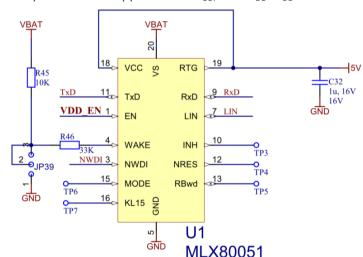
To supply  $V_{DD}$ , the MLX80051 is used, see Figure 4-3. This Melexis System Basis IC provides both LIN transceiver and 5V voltage regulator. The 5V voltage regulator is capable to deliver 70mA and is used to supply VDD to the pre-driver and to supply the microcontroller (MCU). The regulated 5V is decoupled with a 1uF capacitance.
