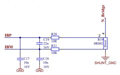
Figure 4-7. Current Sense Input Filter
