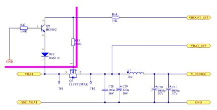
Figure 4-2 Reverse Polarity N-FET and CLC-filter
