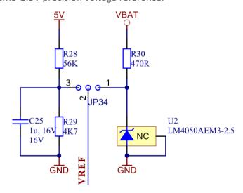
Figure 4-8. Current Sense Output Bias Voltage
