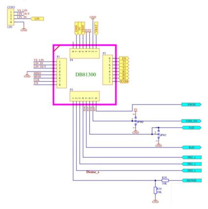
Figure 4-9 Microcontroller Connection
