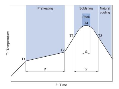
Preheating Soldering Peak Temp. Time Temp. Time Temp. Time **T1** T2 **T**4 t1 тз t2 t3 150°C 180°C 60 to 120s 220°C 40s 260°C 5s
