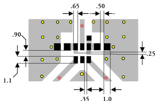
\* Line width should be designed to provide 50 $\Omega$  impedance matching characteristics.
