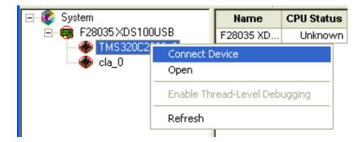
8. This step applies ONLY to Piccolo F28035 users. Once the C28x CPU or CLA is connected you can now launch the CCS debugging window under the Open menu.
