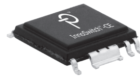
Figure 2. High Creepage, Safety-Compliant eSOP Package.
