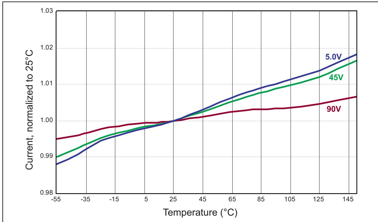
**FIGURE 3-2:** Temperature Characteristics
