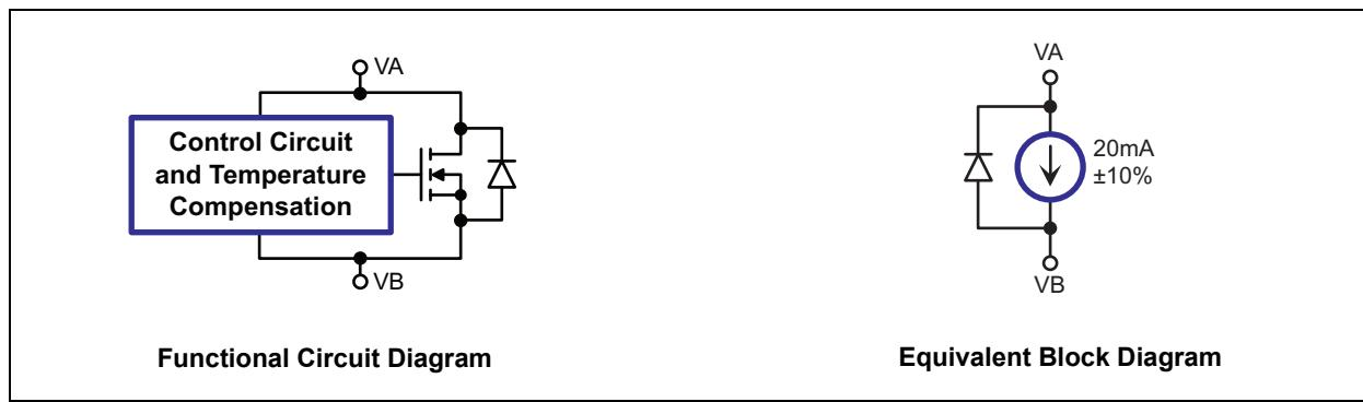
**FIGURE 3-1:** Functional Circuit Diagram and Equivalent Block Diagram
