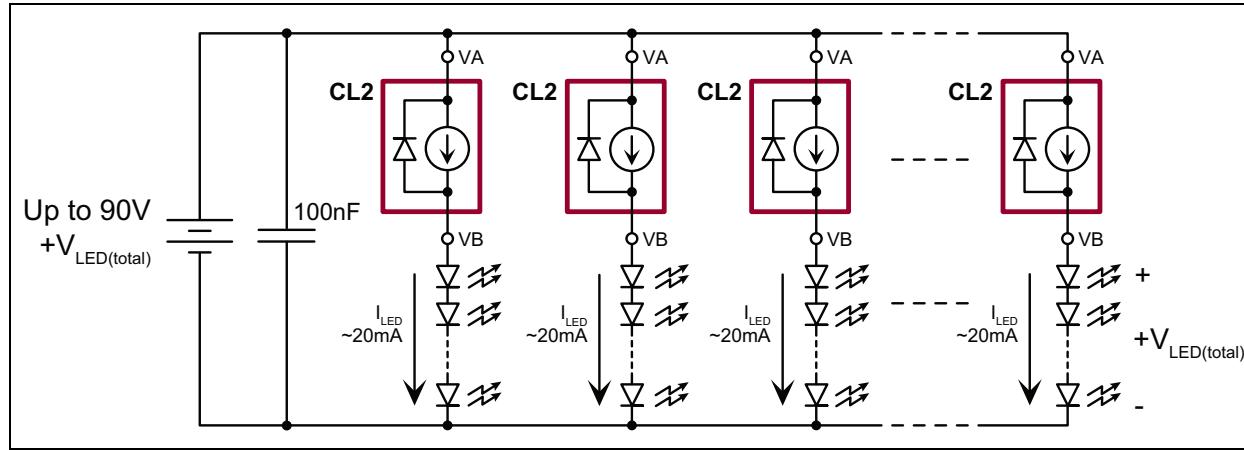
**FIGURE 3-4:** CL2 for Multiple LED Strings
